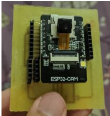
Figure 2 : The ESP-32 camera shield circuit fabricated on the Printed Circuit Board (PCB).
