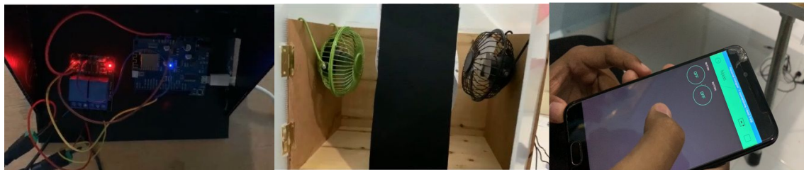
Figure 2: Connection of Paper Dryer Box (left), Inside the Paper Dryer Box (middle), Blynk Application (right)
