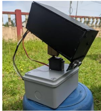
Figure 3 : Prototype of 360 camera surveillance using Iot.
