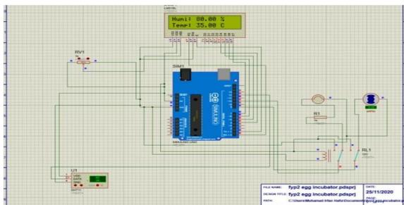
Figure 2. Smart egg incubator circuit diagram
