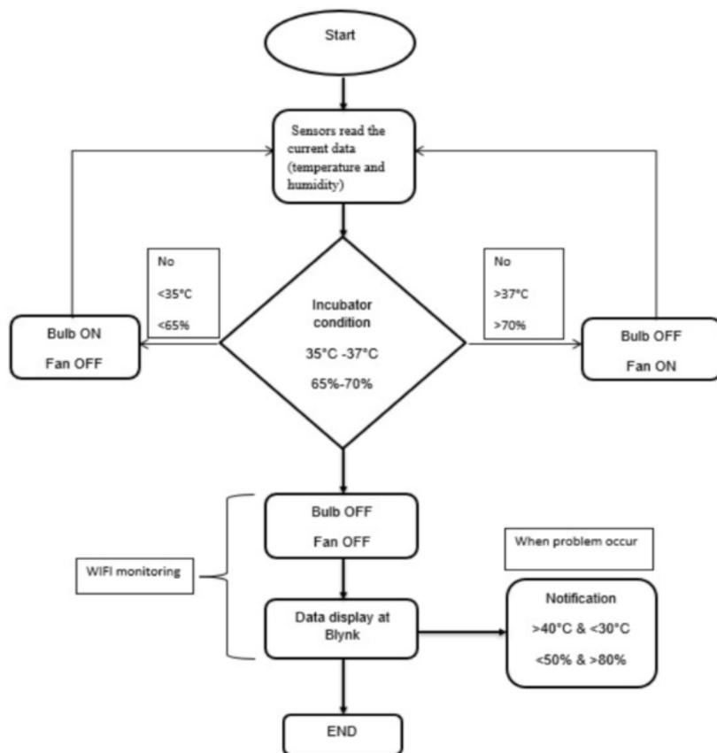
Figure 1. Block diagram of this project
