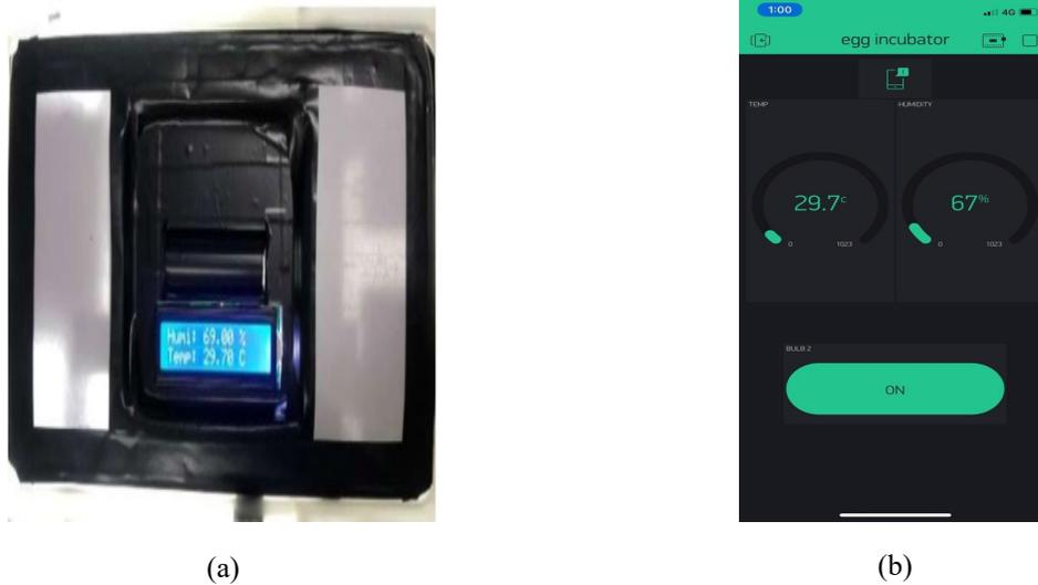
Figure 4: (a) Temperature and humidity data on LCD display, (b) Temperature and humidity data on Blynk app using smartphone
