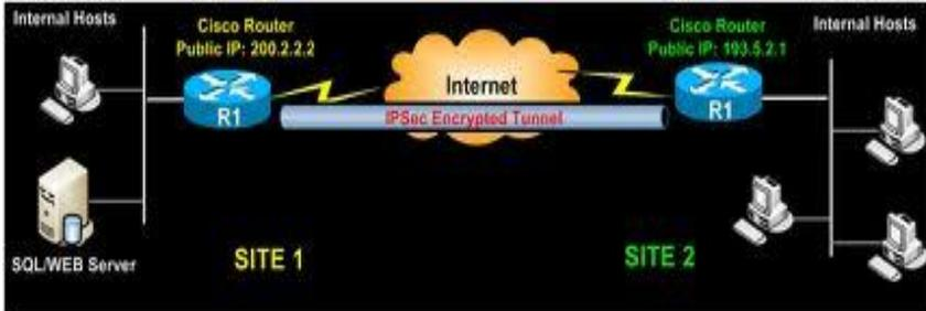
Figure 5.15: VPN configuration (VPN between two Internet sites)
