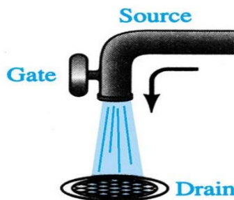
Figure 4.3: Water Spigot vs JFET Operation
