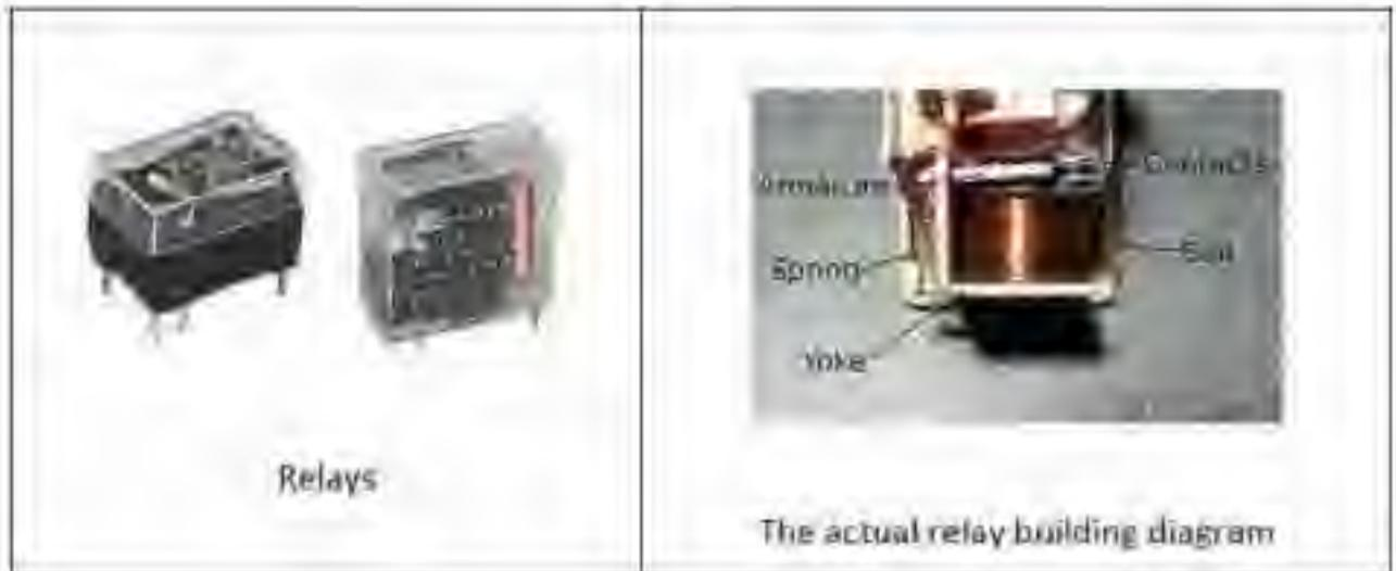
A simple electromagnetic relay consists of a coil of wire wrapped around a soft iron core, an iron yoke which provides a low reluctance path for magnetic flux, a movable iron armature, and one or more sets of contacts. The armature is hinged to the yoke and mechanically linked to one or more sets of moving contacts. It is held in place by a spring so that when the relay is de-energized there is an air gap in the magnetic circuit.
