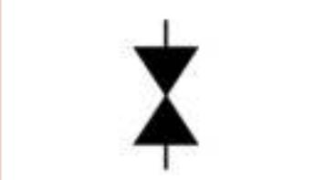
The symbol for a Gunn diode is a black vertical line with two triangles pointing towards each other in the center, forming a narrow waist.                                                                                                                                                                                                                                      |
