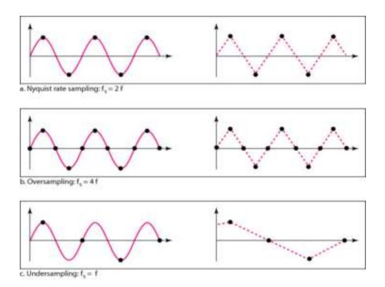
Figure 2.25: Recovery of A Sampled Sine Wave for Different Sampling Rates
