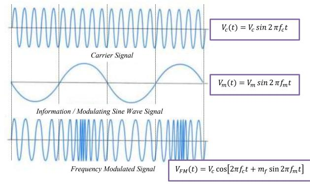
Figure 2.9: FM Generation Using FM Modulator
