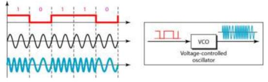
Figure 2.34: Binary Frequency Shift Keying (FSK)
