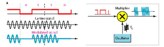
Figure 2.33: Binary Amplitude Shift Keying (ASK)
