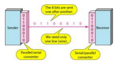
Figure 4.7: Serial Data Transmission
