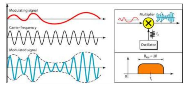
Figure 2.7: Multi-Frequency Amplitude Modulation
