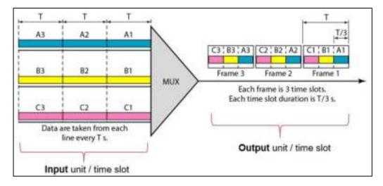
Figure 3.5: Synchronous time-division multiplexing
