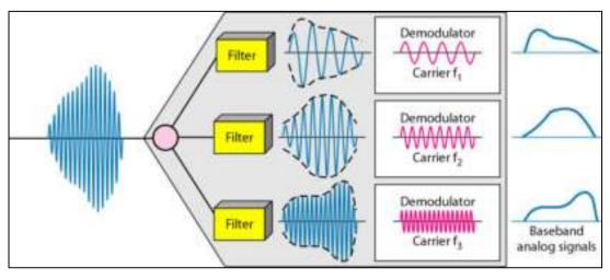
Figure 3.10: FDM Demultiplexing Process
