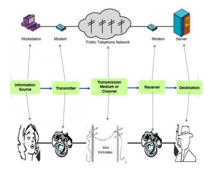
Figure 1.2: Telephony Communication System Block Diagram
