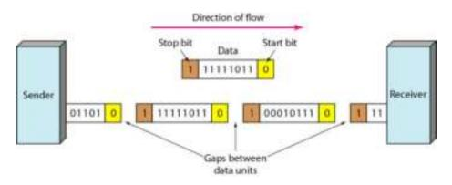
Figure 4.8: Asynchronous Transmission
