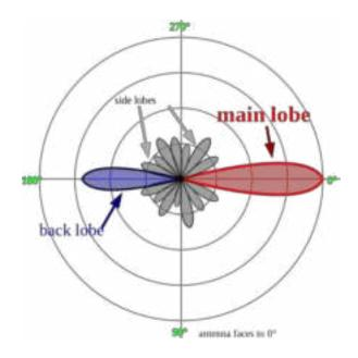
Figure 3.34: Radiation Pattern of Antenna
