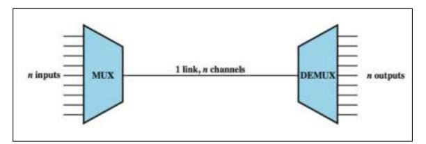
Figure 3.1: Multiplexing & Demultiplexing
