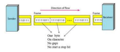
Figure 4.9: Synchronous Transmission
