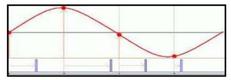
Figure 2.15: Pulse Position Modulation (PPM)
