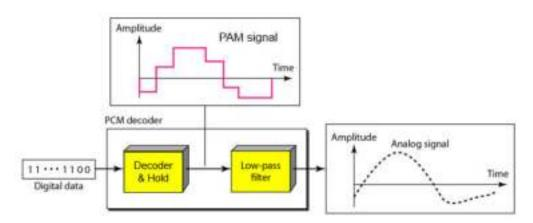
Figure 2.29: Block Diagram of PCM Decoder (Receiver)
