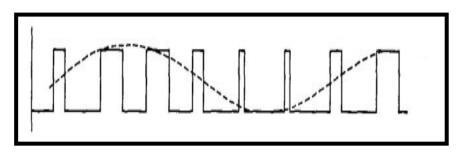
Figure 2.14: Pulse Width Modulation (PWM)
