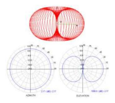
Figure 3.36: Omnidirectional Radiation Pattern
