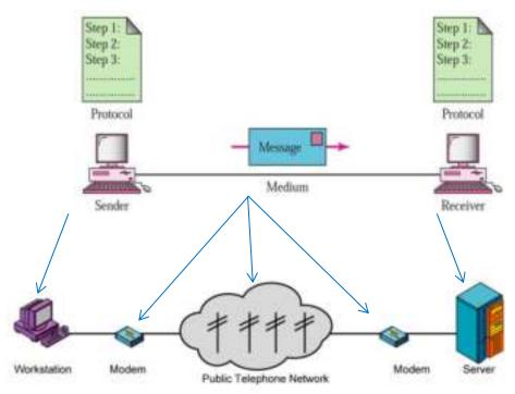
Figure 1.20: Block Diagram of Data Communication
