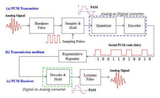
Figure 2.18: Block Diagram of PCM
