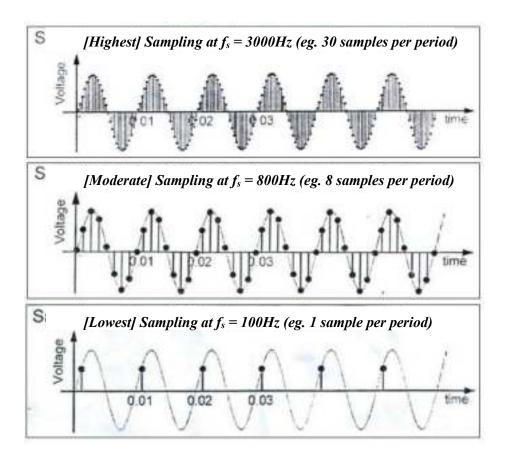
Figure 2.21: Example of Highest, Moderate and Lowest Sampling Rate for PCM
