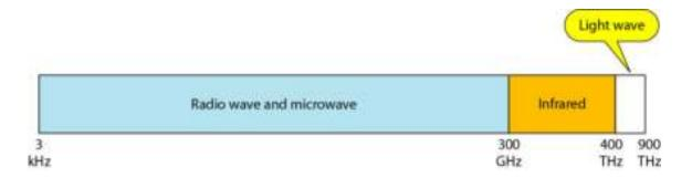
Figure 3.30: Electromagnetic Spectrum for Wireless Communication
