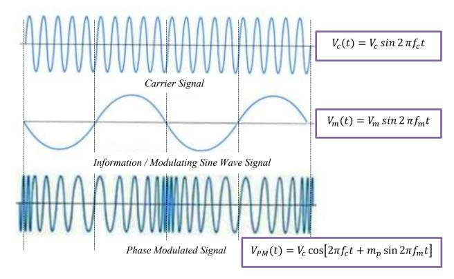
Figure 2.10: PM Generation Using PM Modulator
