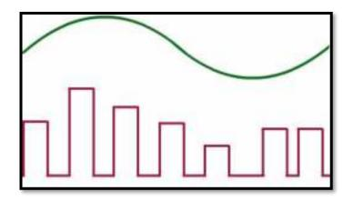
Figure 2.16: Pulse Amplitude Modulation (PAM)
