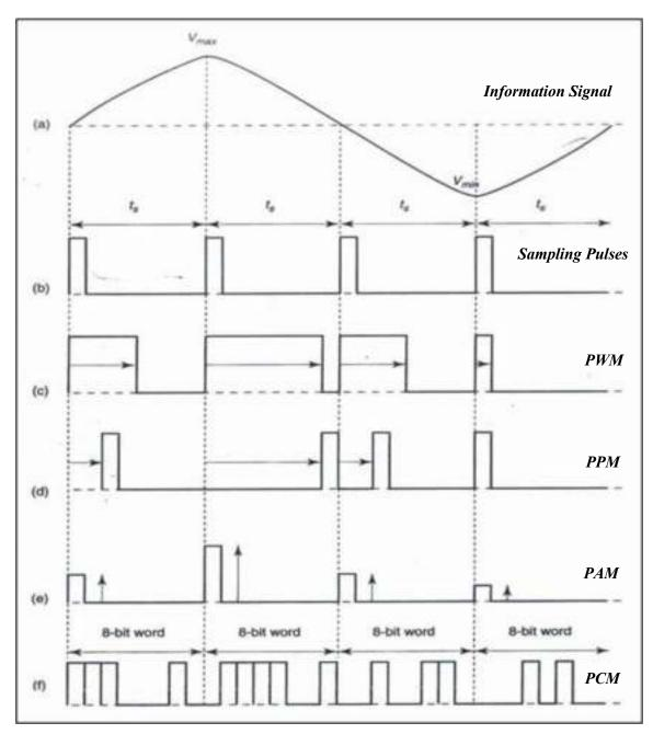
Figure 2.17: Pulse Modulation Technique
