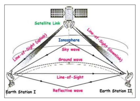
Figure 3.31: Radio Waves Propagation
