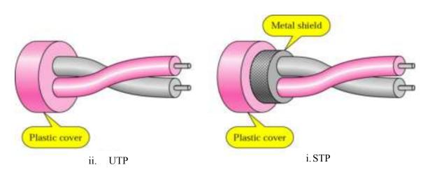
Figure 3.16: Types of Twisted Pair Cable
