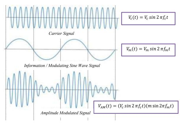
Figure 2.5: AM Generation Using non-liner AM Modulator
