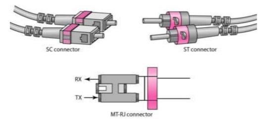
Figure 3.23: Fiber Optic Cable Connectors
