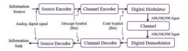
Figure 2.12: Basic Elements of Digital Communication System
