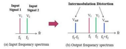
Figure 1.8: Intermodulation Distortion
