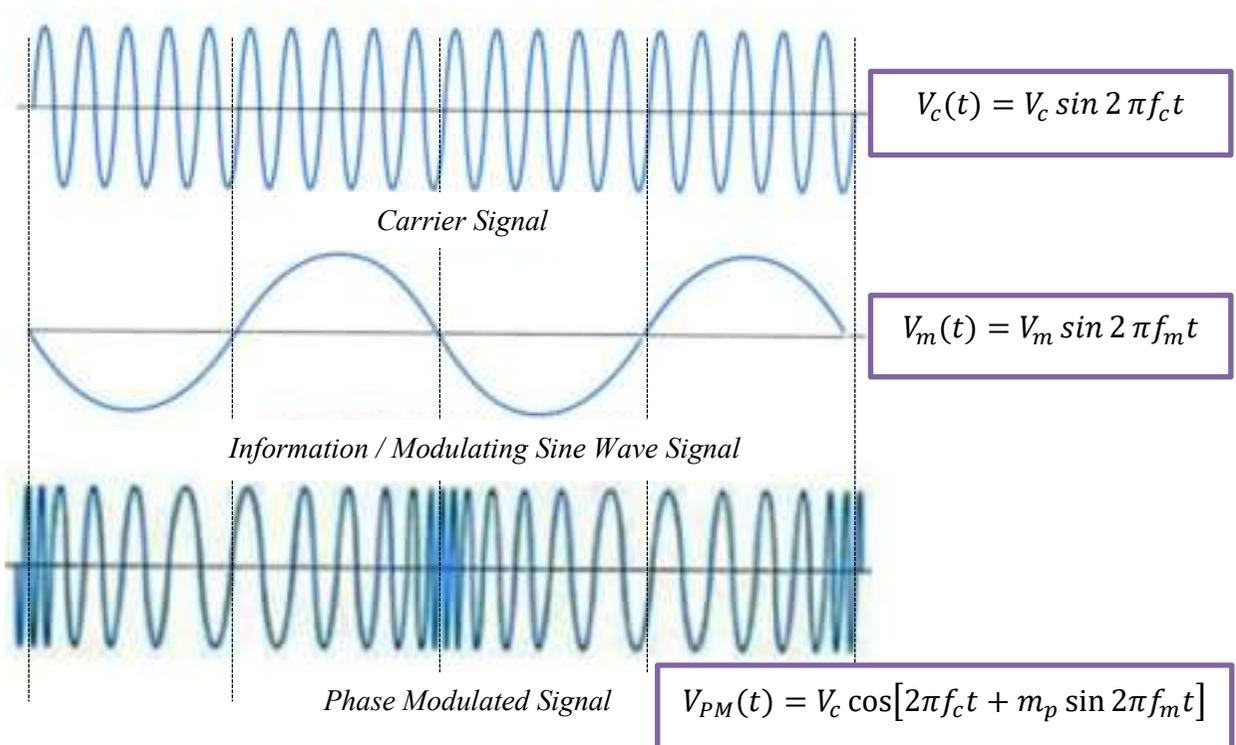
Figure 2.10: PM Generation Using PM Modulator
