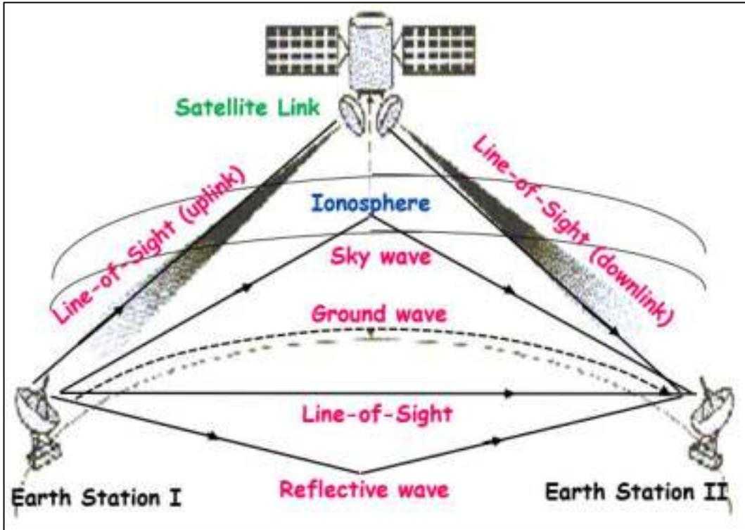
Figure 3.31: Radio Waves Propagation
