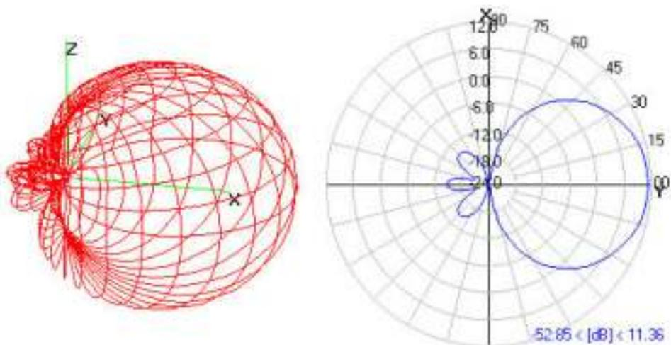
Figure 3.38: Directional Radiation Pattern
