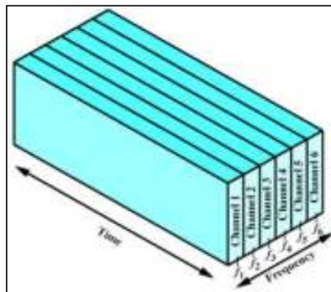
Figure 3.7: FDM Communication Resources (CR) Allocation
