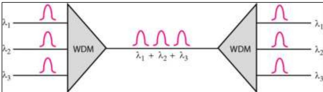
Figure 3.11: Wavelength-division multiplexing (WDM)
