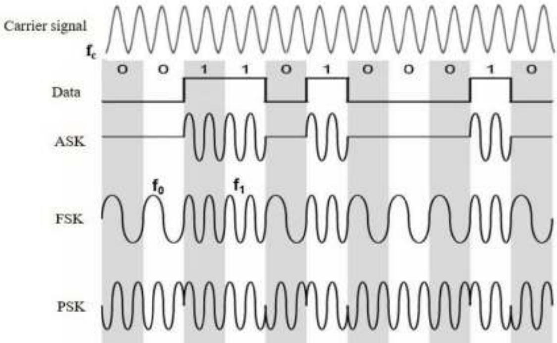
Figure 2.32: Digital Modulation Techniques
