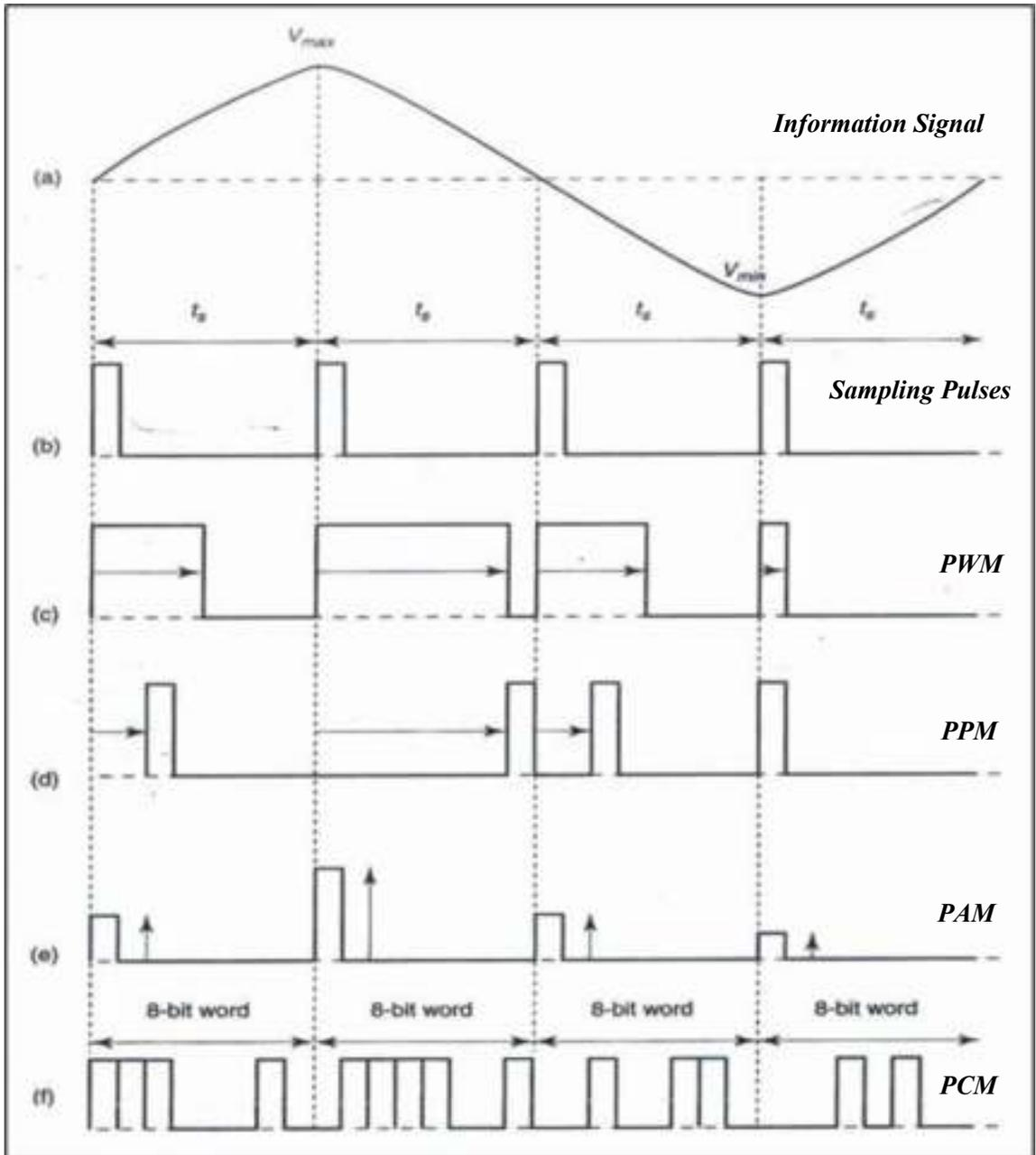
Figure 2.17: Pulse Modulation Technique
