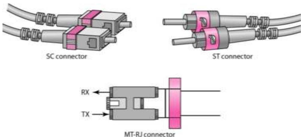
Figure 3.23: Fiber Optic Cable Connectors
