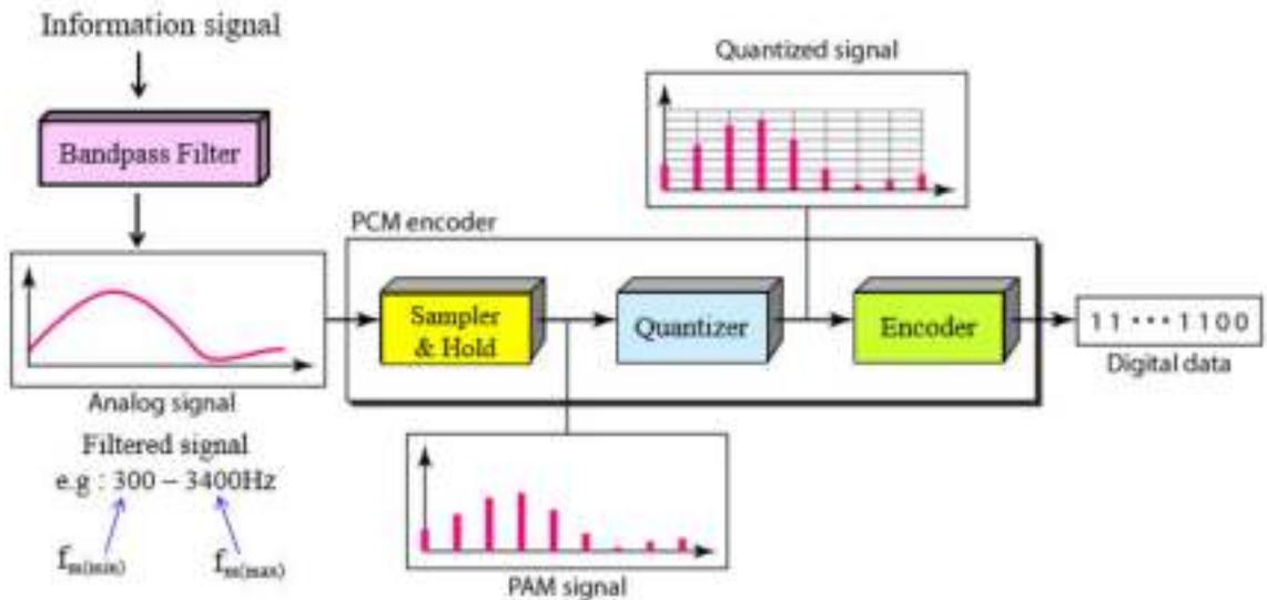
Figure 2.19: Block Diagram of PCM Encoder (Transmitter)
