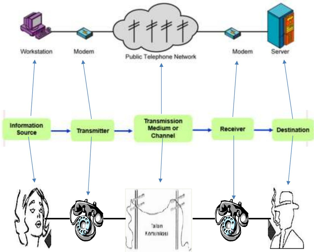
Figure 1.2: Telephony Communication System Block Diagram
