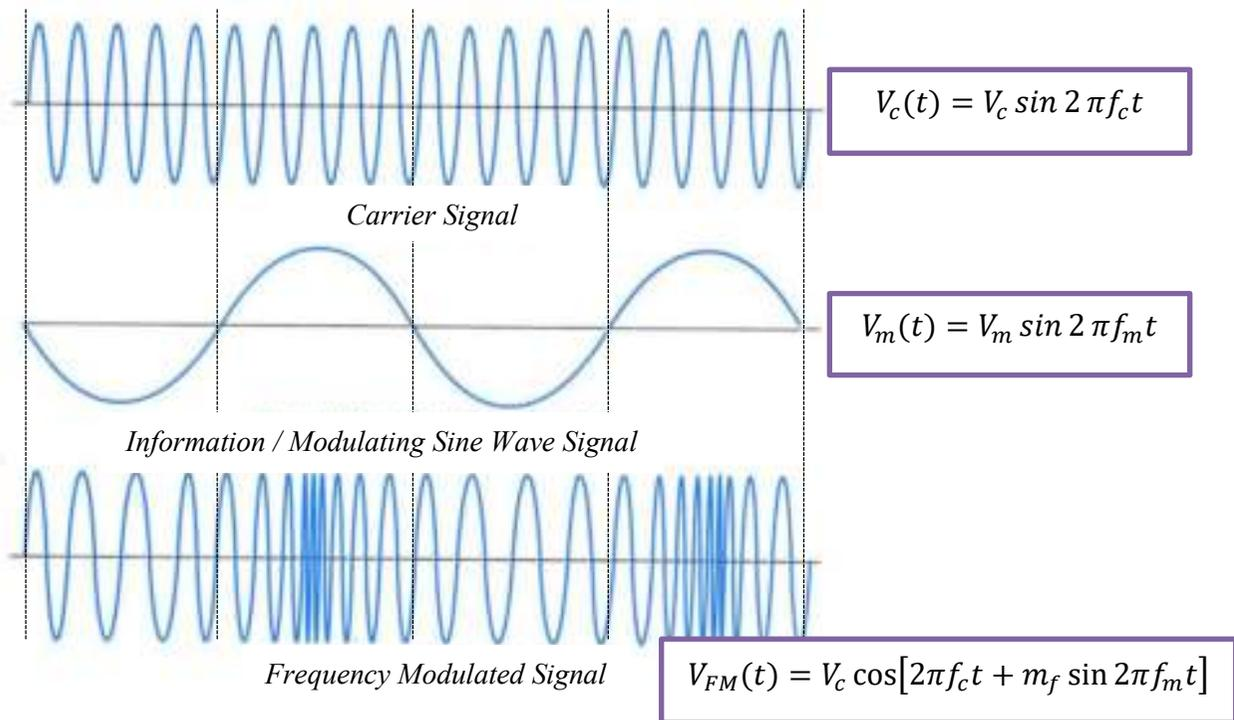
Figure 2.9: FM Generation Using FM Modulator
