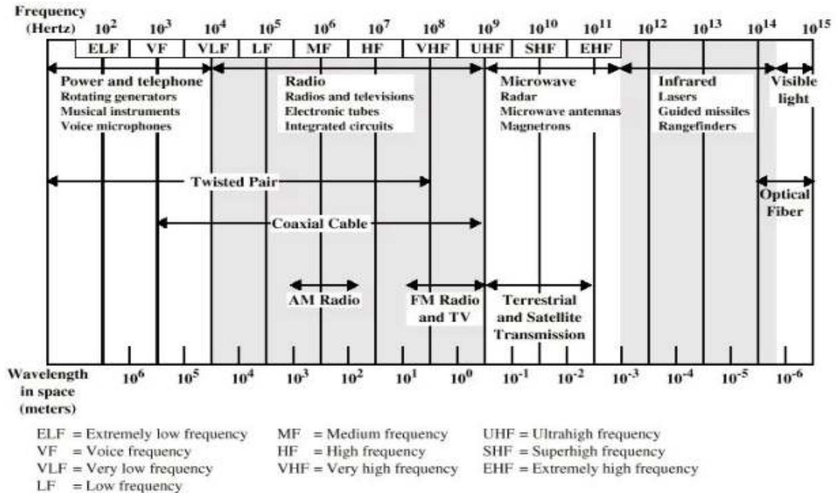
Figure 1.10: Frequency Spectrum
