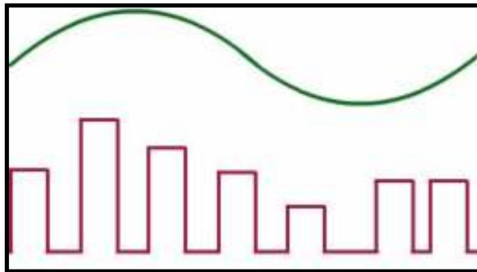
Figure 2.16: Pulse Amplitude Modulation (PAM)
