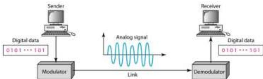
Figure 2.30: Digital-to-analog conversion
