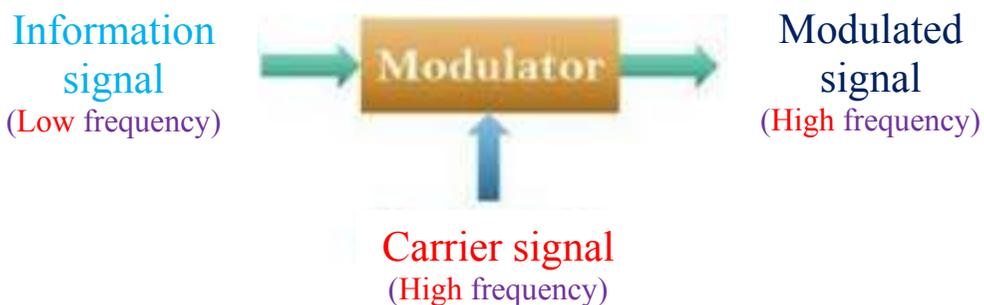
Figure 2.1: Modulation Process
