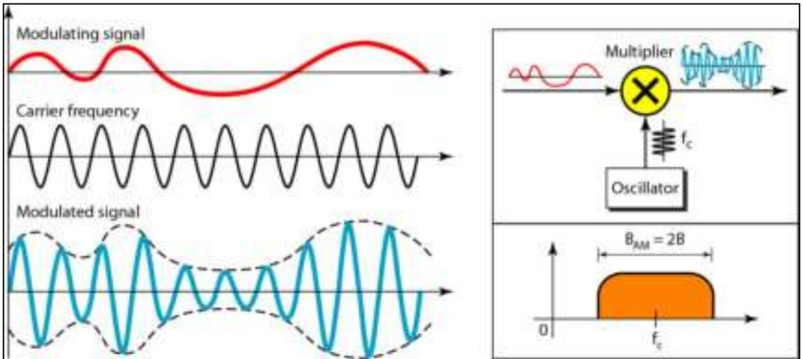
Figure 2.7: Multi-Frequency Amplitude Modulation
