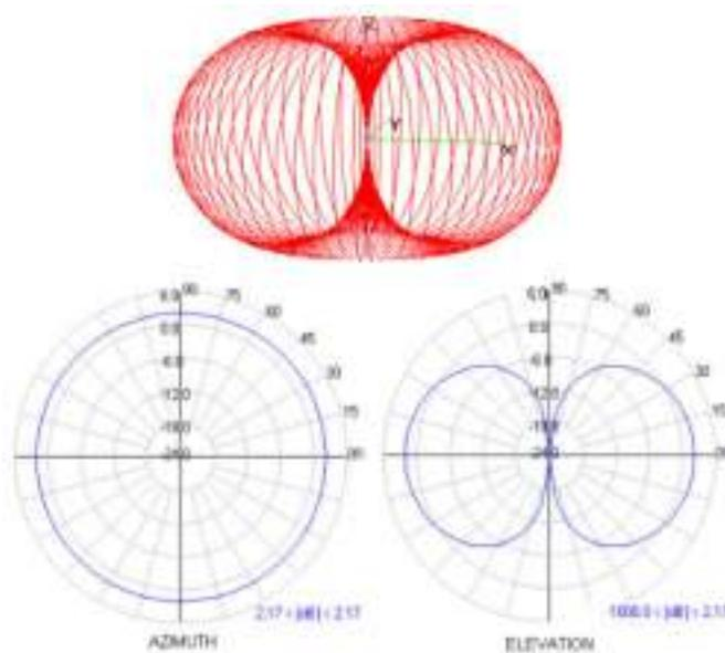
Figure 3.36: Omnidirectional Radiation Pattern
