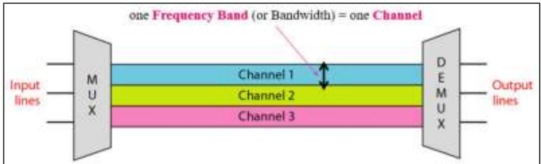
Figure 3.6: Frequency Division Multiplexing (FDM)
