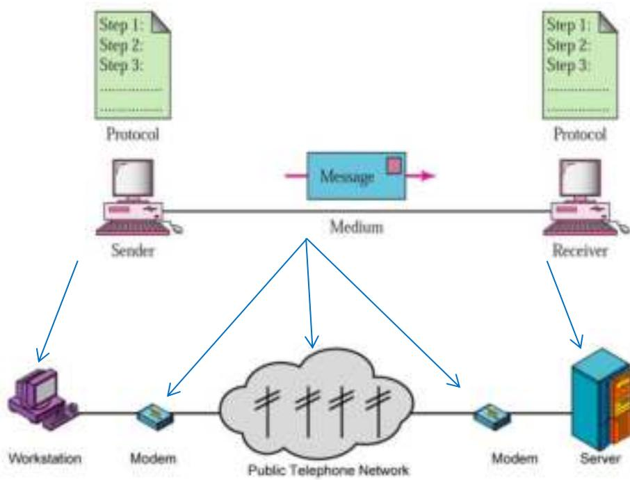
Figure 1.20: Block Diagram of Data Communication
