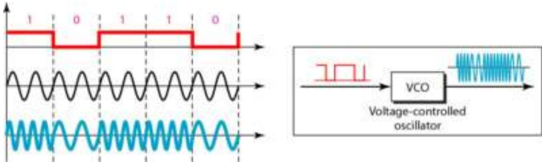
Figure 2.34: Binary Frequency Shift Keying (FSK)
