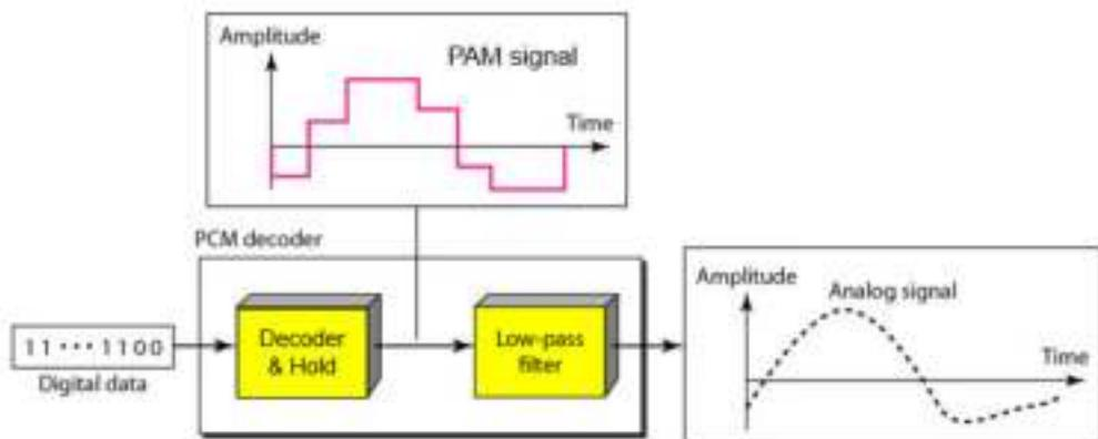
Figure 2.29: Block Diagram of PCM Decoder (Receiver)
