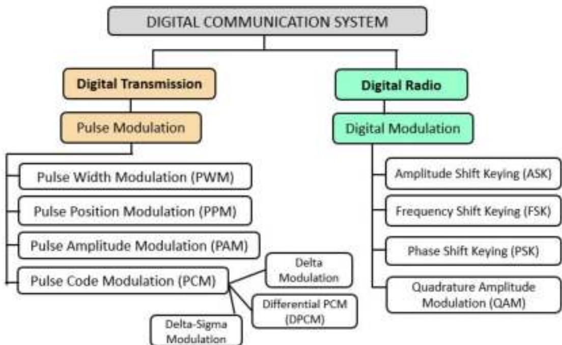
Figure 2.11: Types of Digital Communication
