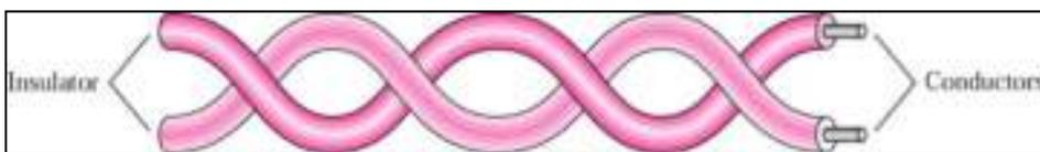
Figure 3.15: Twisted Pair Cable
