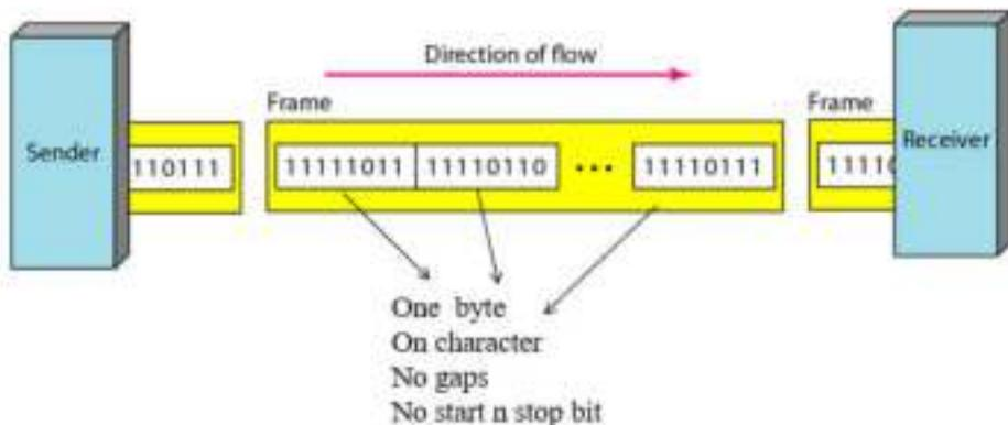
Figure 4.9: Synchronous Transmission
