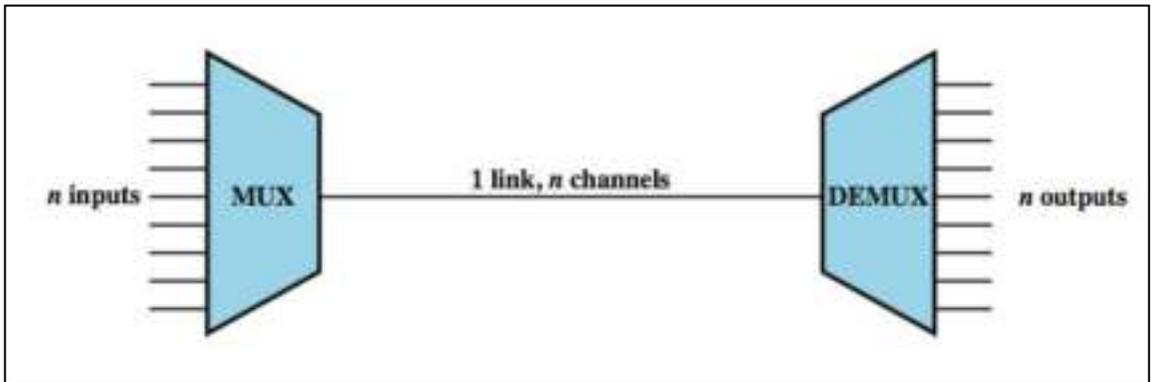
Figure 3.1: Multiplexing & Demultiplexing
