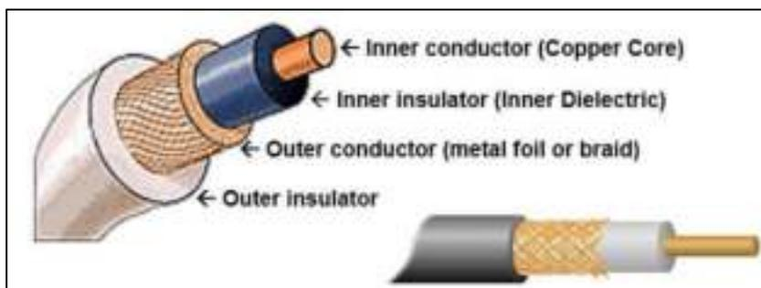
Figure 3.18: Structure of Coaxial Cable
