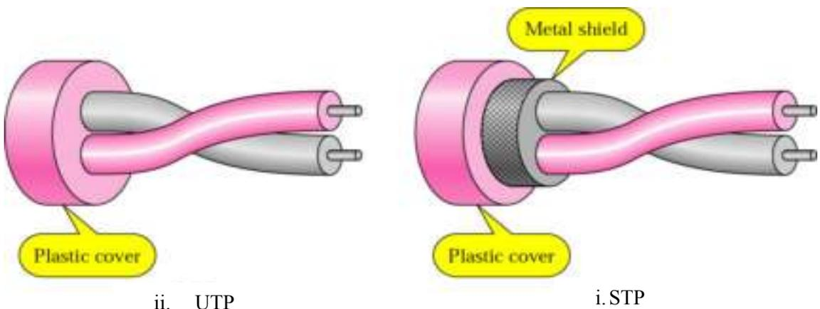
Figure 3.16: Types of Twisted Pair Cable
