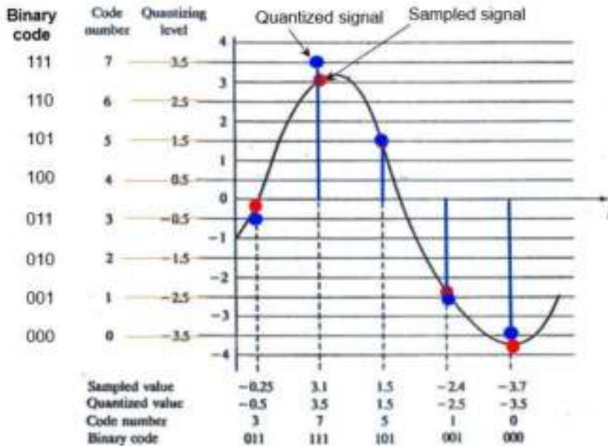
Figure 2.28: The essential features of binary PCM
