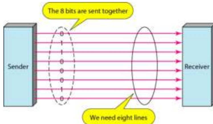
Figure 4.6: Parallel Data Transmission
