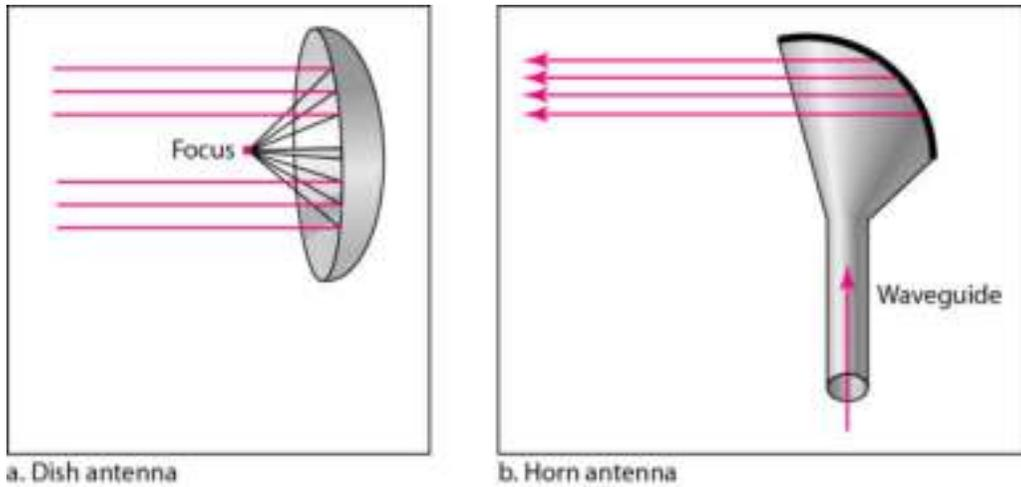
Figure 3.37: Directional Antenna
