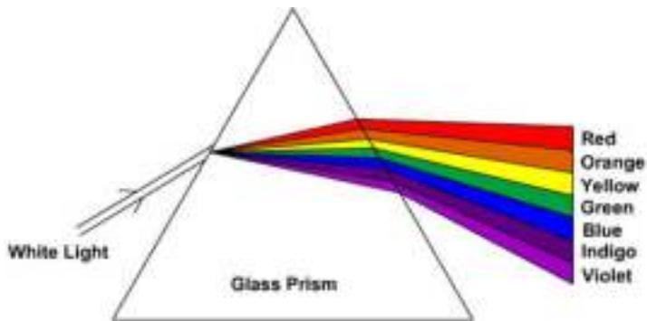
Figure 3.13: Dispersion of light by Glass Prism
