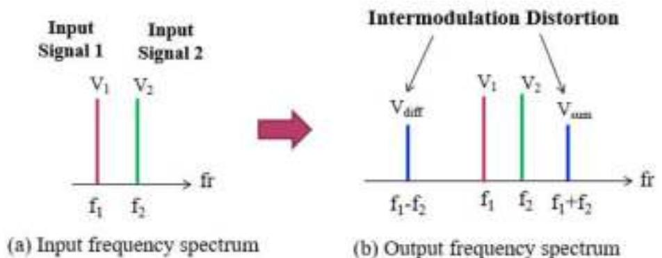
Figure 1.8: Intermodulation Distortion
