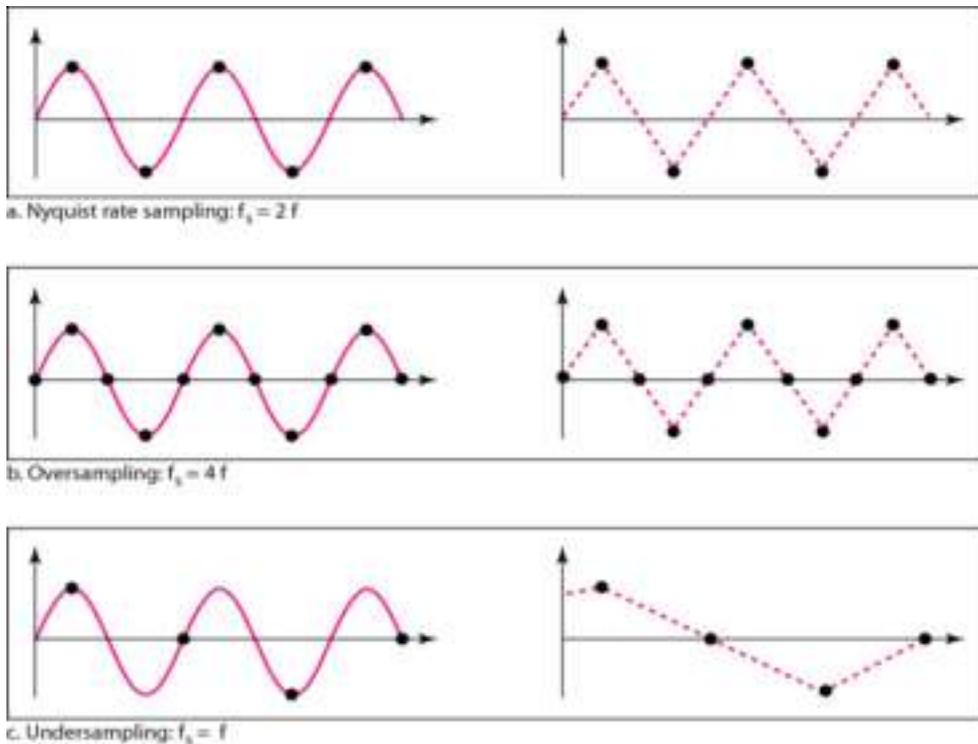
Figure 2.25: Recovery of A Sampled Sine Wave for Different Sampling Rates
