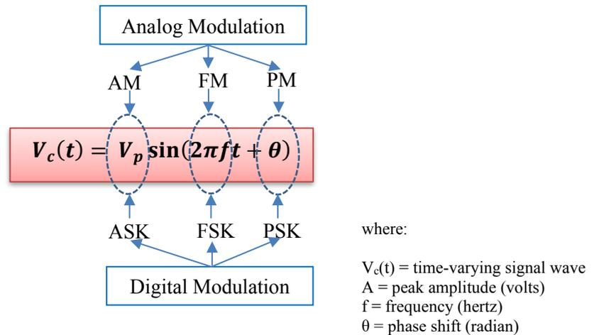
Figure 2.4: General Equation for Modulation Technique
