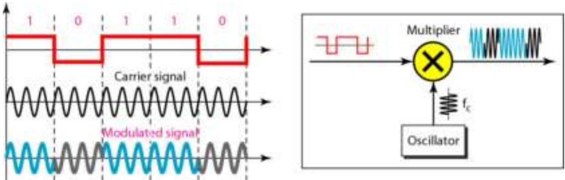
Figure 2.35: Binary Phase Shift Keying (PSK)
