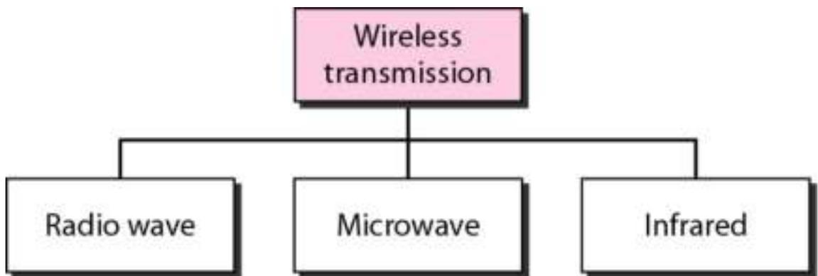
Figure 3.29: Wireless Transmission
