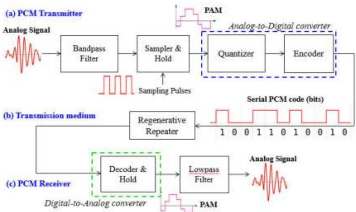
Figure 2.18: Block Diagram of PCM
