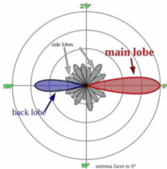
Figure 3.34: Radiation Pattern of Antenna
