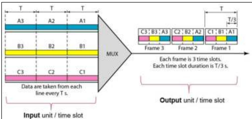
Figure 3.5: Synchronous time-division multiplexing
