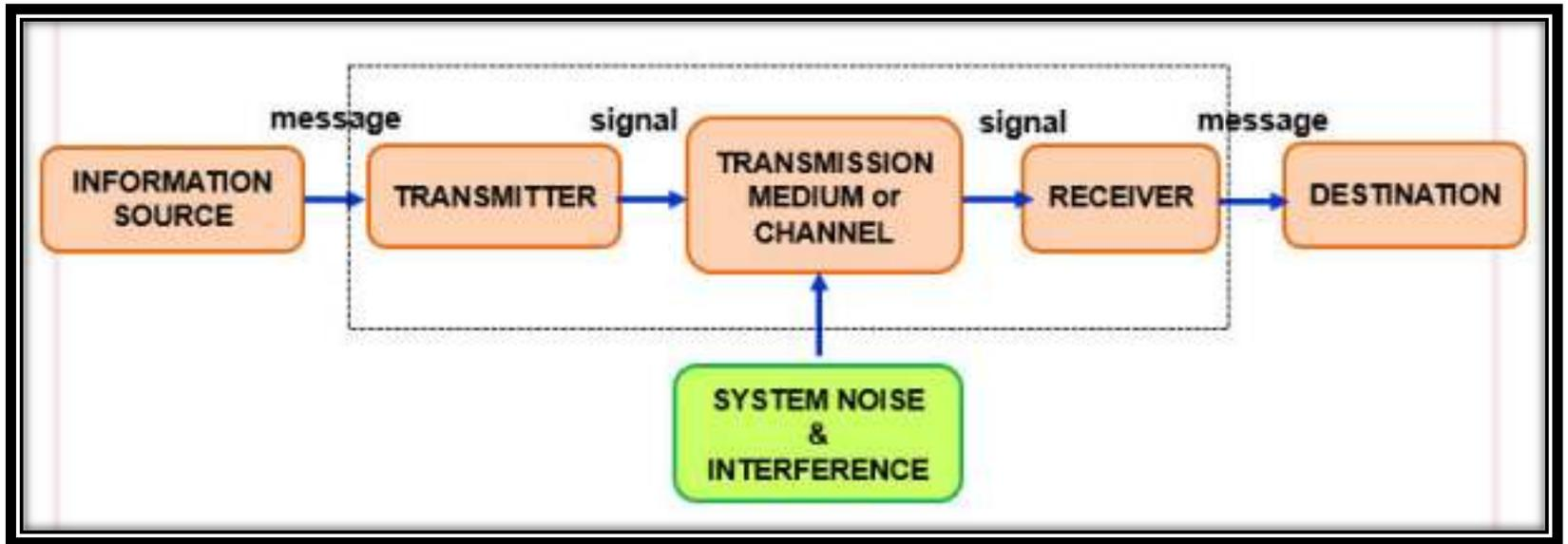
Figure 1.1: Shannon's Basic Block Diagram of an Electronic Communication System
