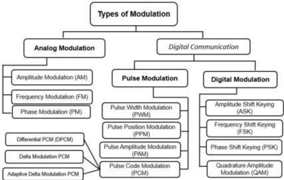
Figure 2.3: Types of Modulation
