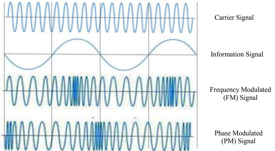
Figure 2.8: Angle Modulation
