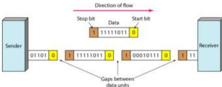
Figure 4.8: Asynchronous Transmission
