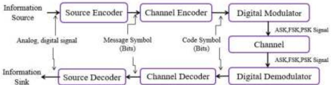
Figure 2.12: Basic Elements of Digital Communication System
