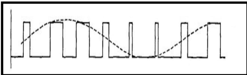
Figure 2.14: Pulse Width Modulation (PWM)
