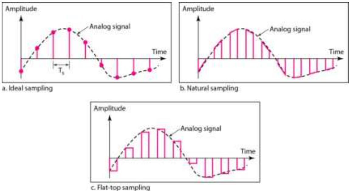
Figure 2.22: Three different sampling methods for PCM
