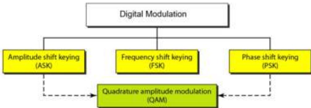
Figure 2.31: Types of Digital Modulation
