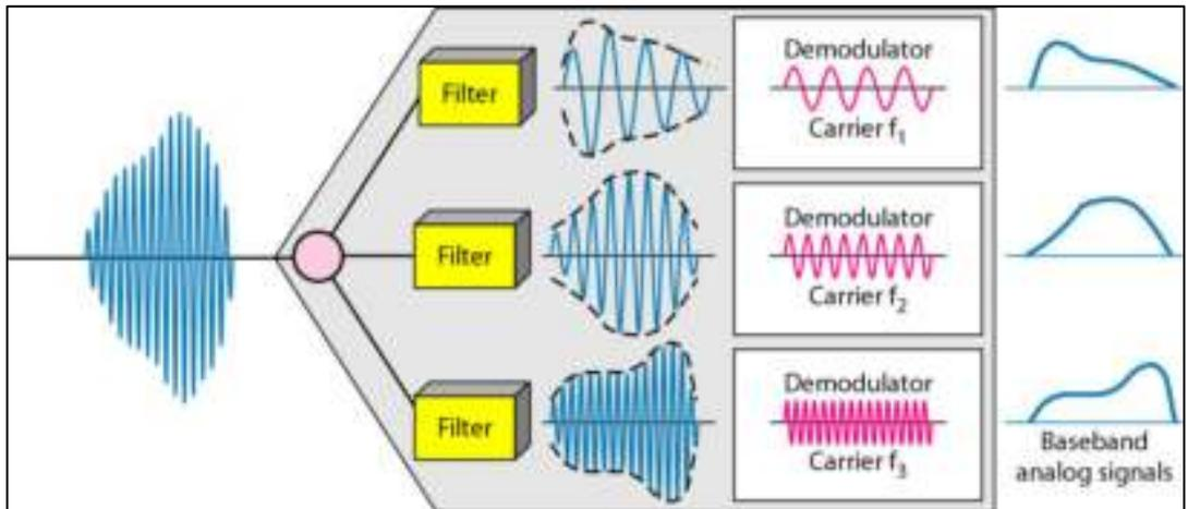
Figure 3.10: FDM Demultiplexing Process
