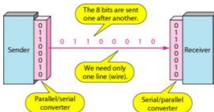
Figure 4.7: Serial Data Transmission
