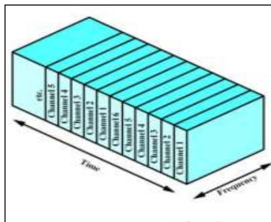
Figure 3.4: TDM Communication Resources (CR) Allocation
