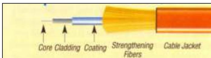
Figure 3.20: Fiber Optic Concentric Sections
