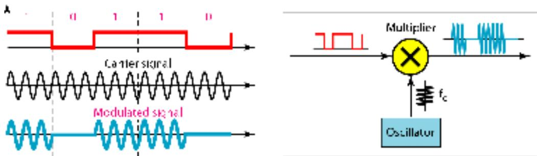
Figure 2.33: Binary Amplitude Shift Keying (ASK)
