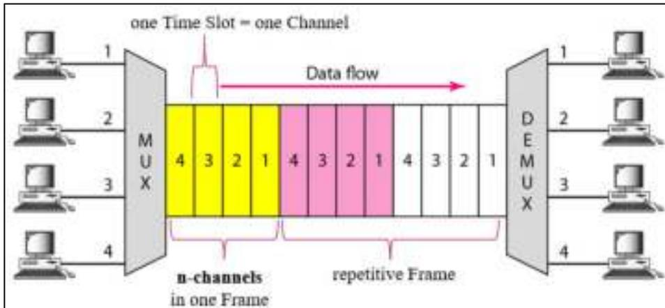
Figure 3.3: Time Division Multiplexing (TDM)
