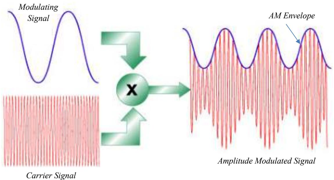
Figure 2.6: Single-Frequency Amplitude Modulation
