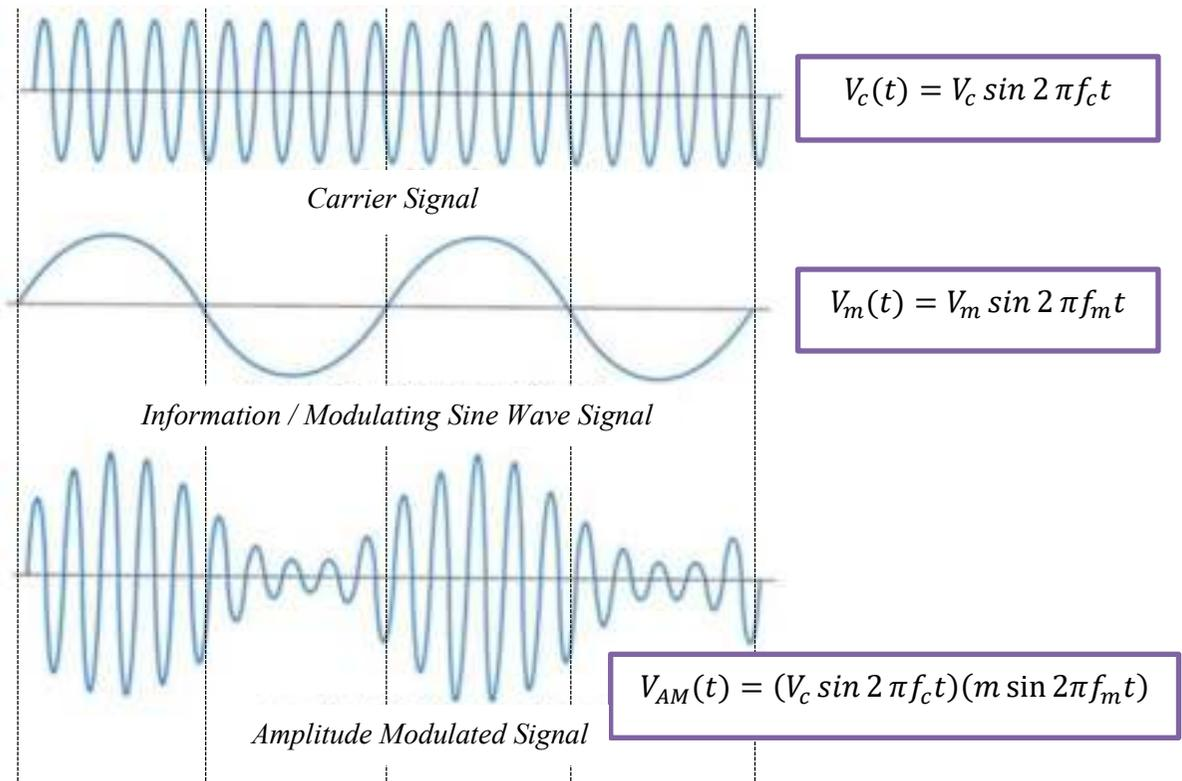
Figure 2.5: AM Generation Using non-linear AM Modulator
