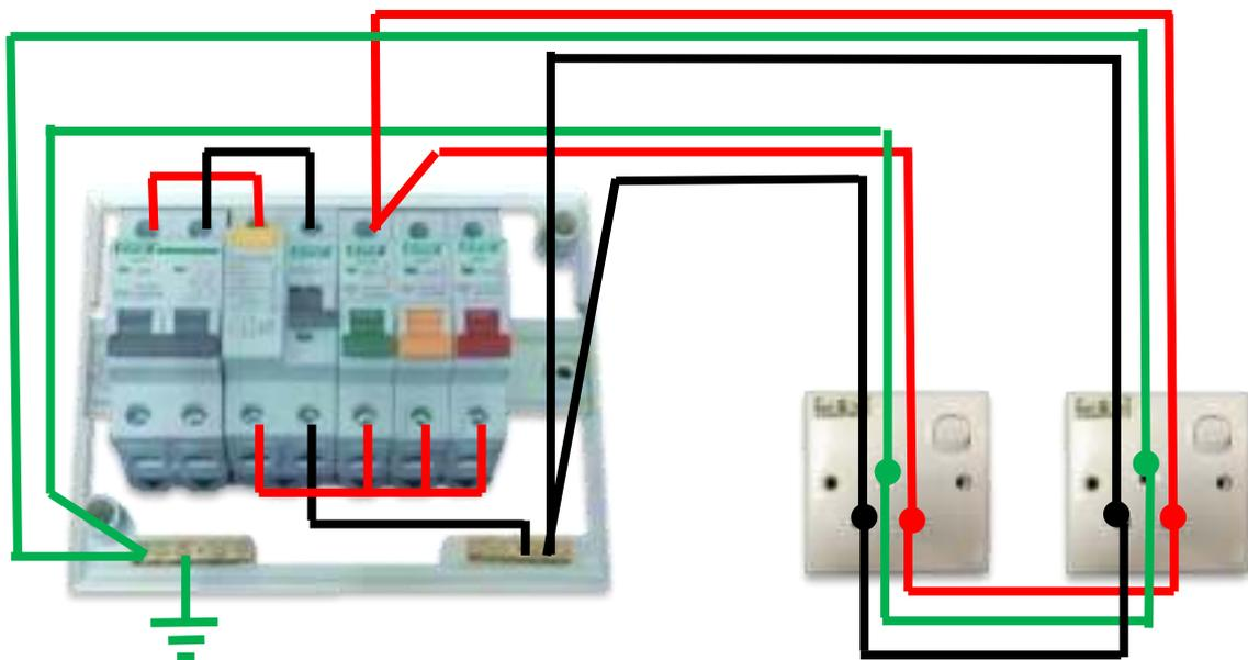
Figure 8: The connection diagram of the power circuit using ring connection
