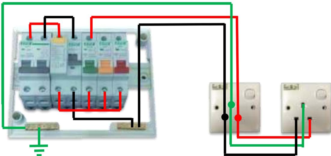
Figure 7: The connection diagram of the power circuit using radial connection
