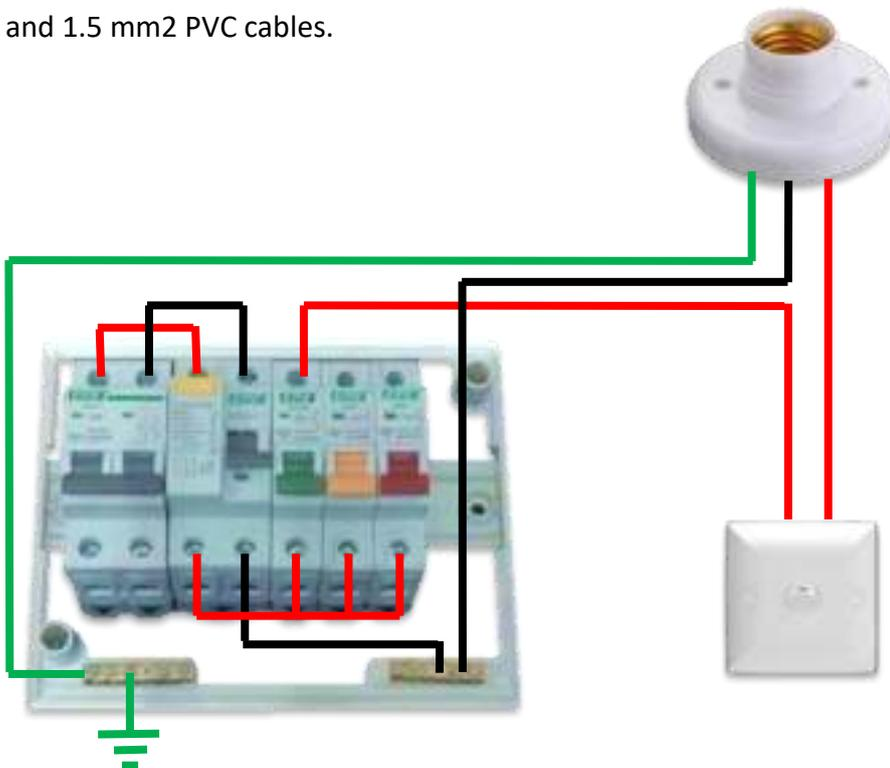
Figure 4: The connection diagram of the light controlled from one point
