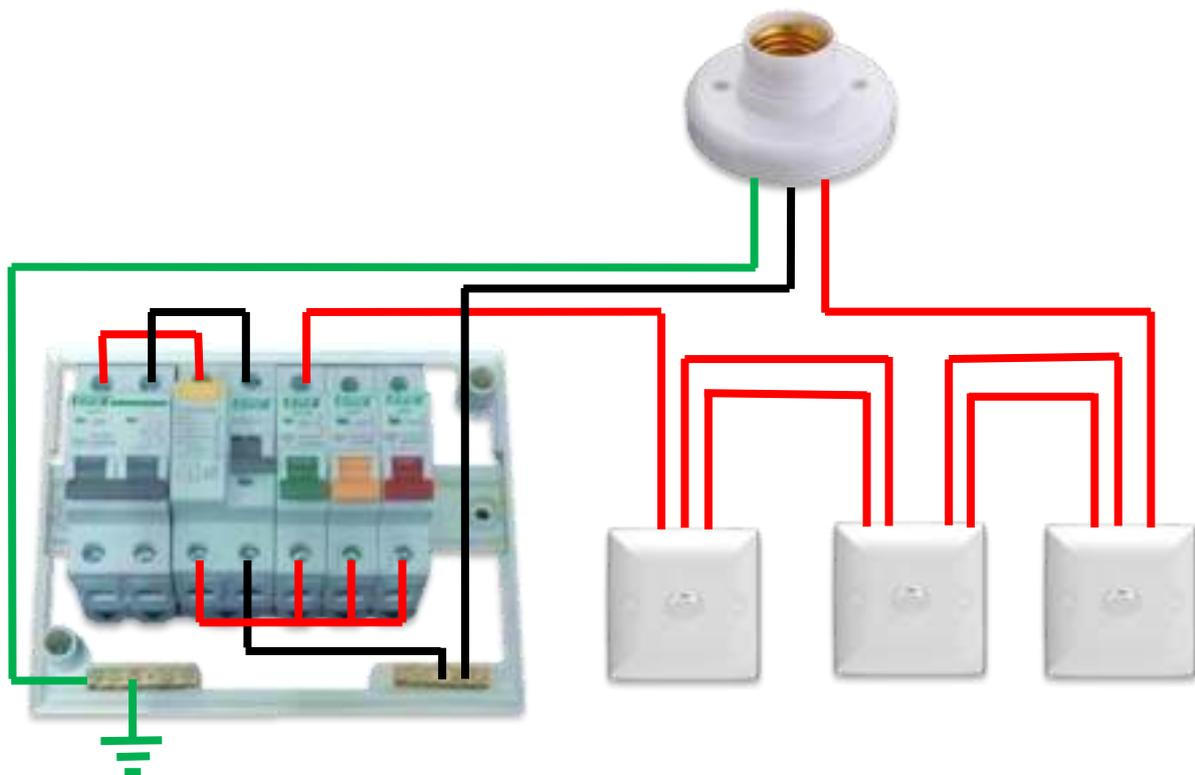
Figure 6: The connection diagram of the light controlled from three points
