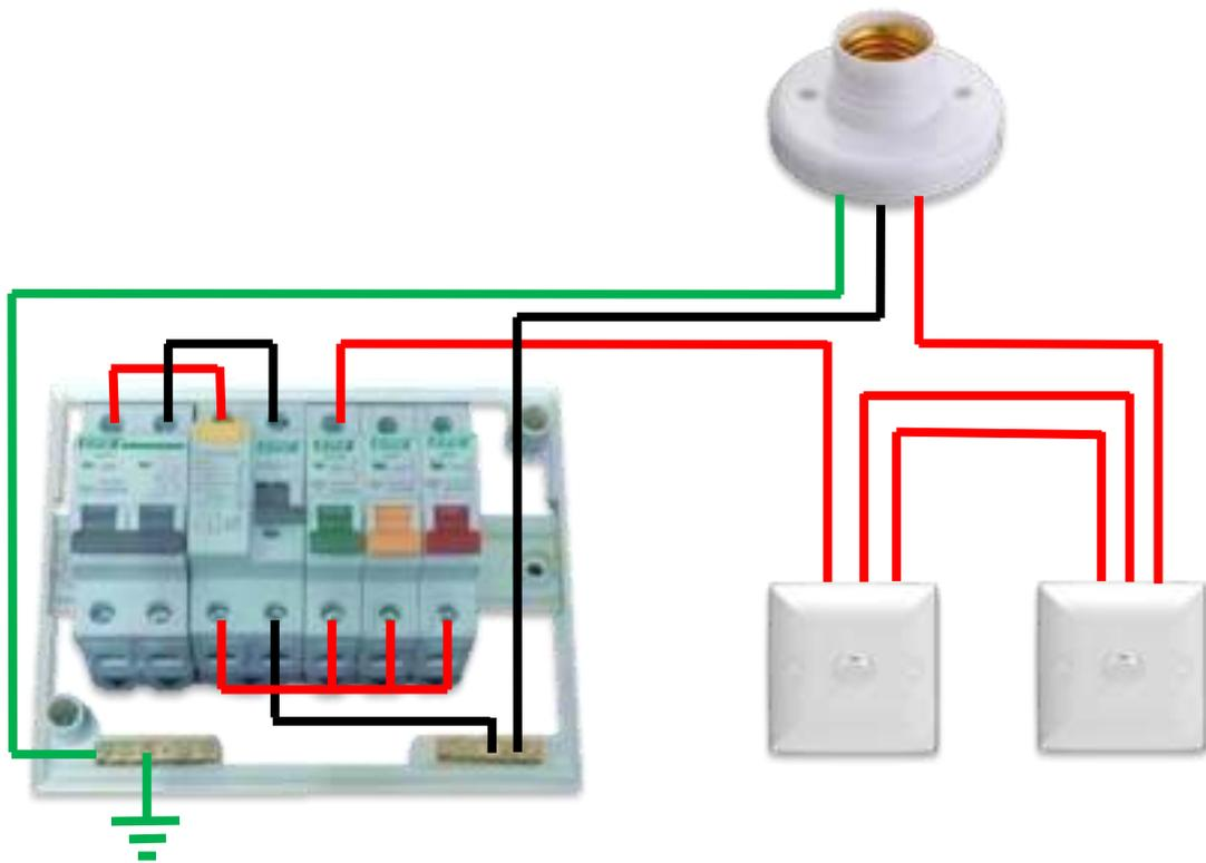
Figure 5: The connection diagram of the light controlled from two points
