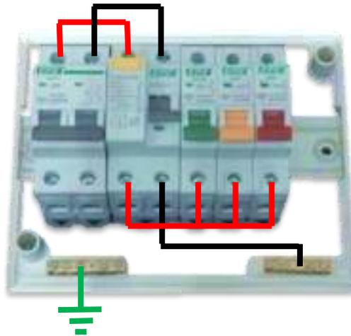
Figure 3: The connection diagram of the main circuit.
