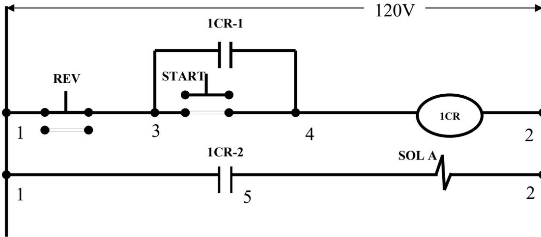
Figure 4.4: Single Solenoid Spring Return Valve.
