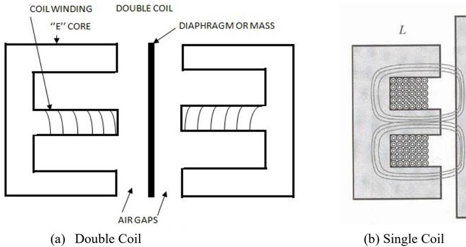
Figure 5.3: Inductive Transducer (htt4)
