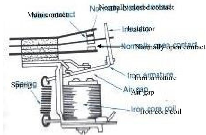
Figure 3.2: Typical physical appearance of a relay
