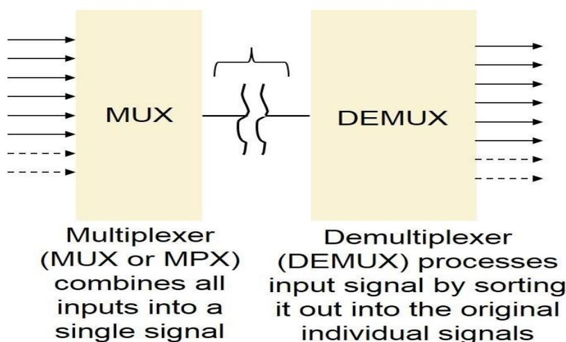
Figure 6.3: Concept of multiplexing.
