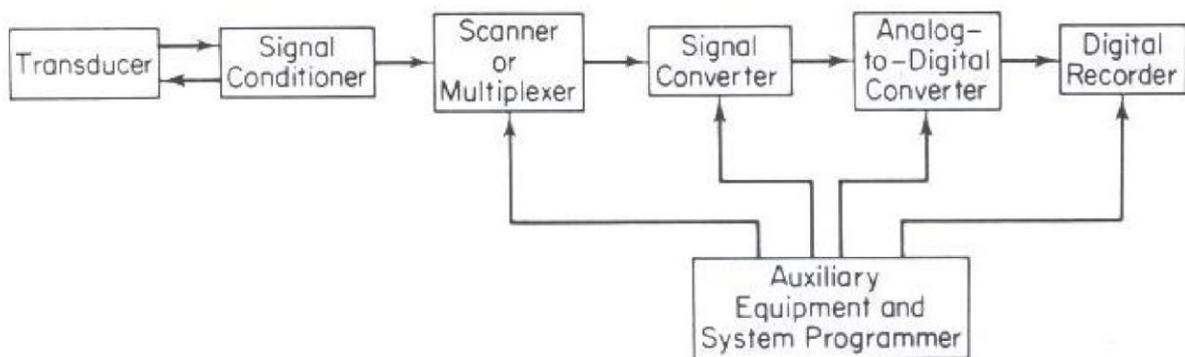
Figure 6.2: Elements of digital data-acquisition system.
