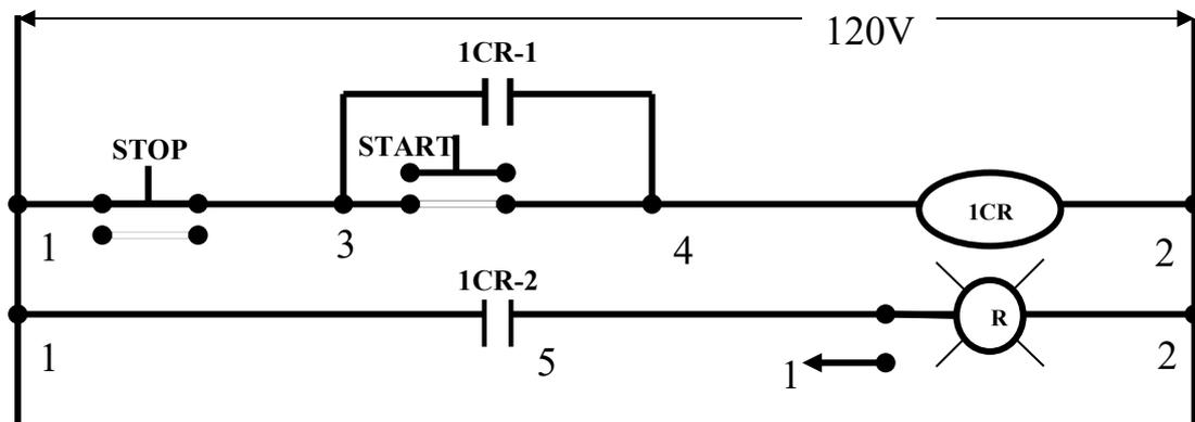
Figure 3.4: A relay with two NO contacts
