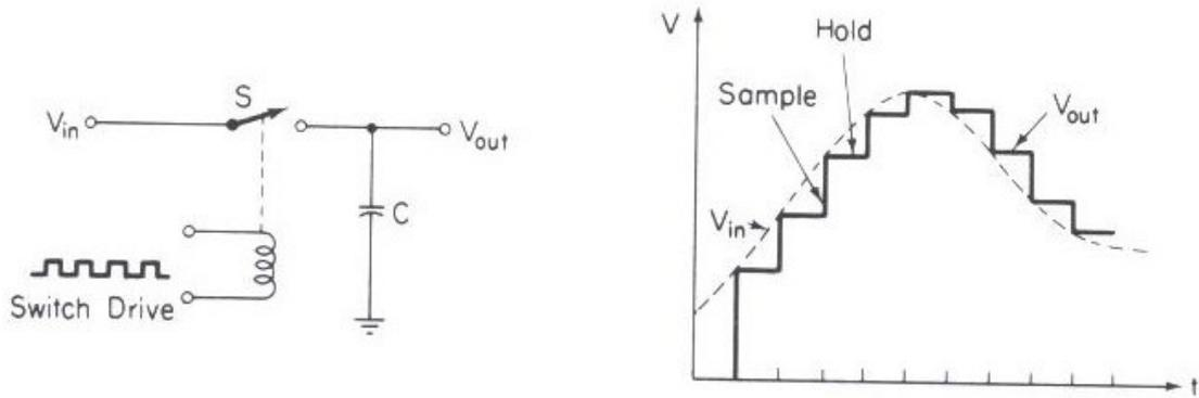
Figure 2.2: Simple sample and Hold circuit
