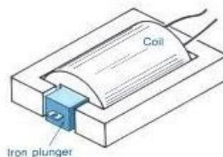
Figure 4.1: Schematic Diagram of Solenoid.
