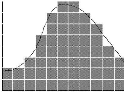
Figure 6.1: Converting the analog to digital signal.
