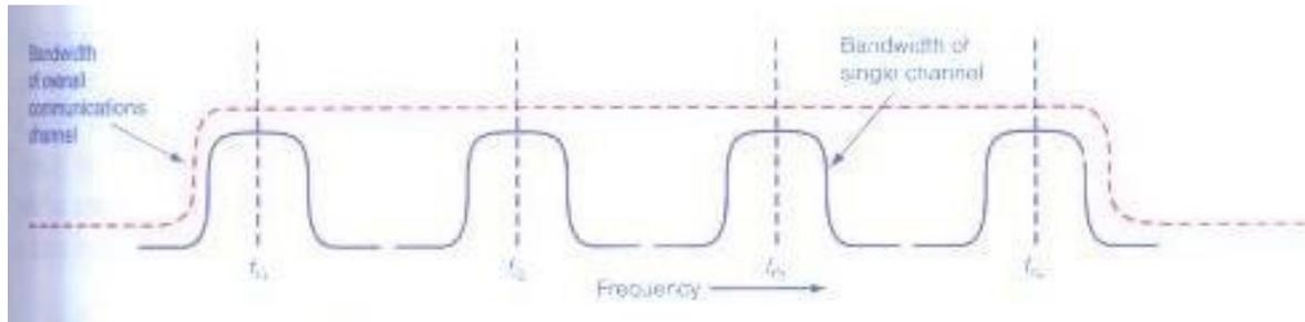
Figure 6.5: Spectrum of an FDM signal.
