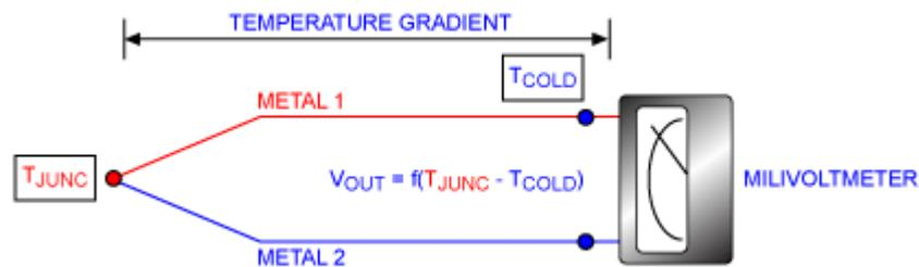
Figure 5.9: Basic Thermocouple Circuit.
