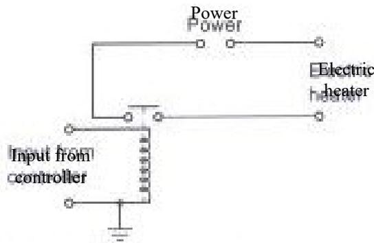
Figure 3.1: Relay Principle
