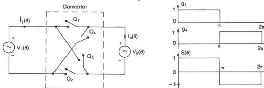
Figure 2.1: Single – phase diagram of converter structure
