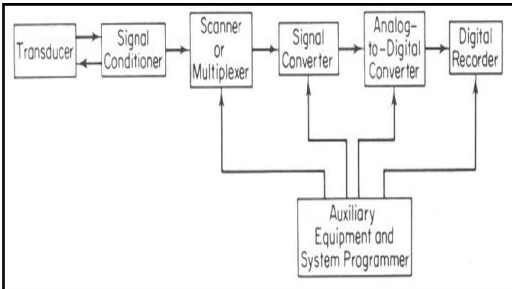
Fig. 1: Elements of digital data-acquisition system
