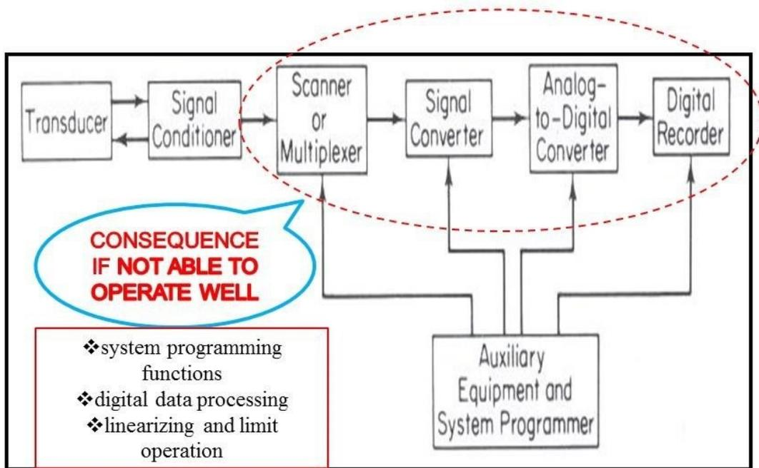
Fig. 1: Elements of digital data-acquisition system
