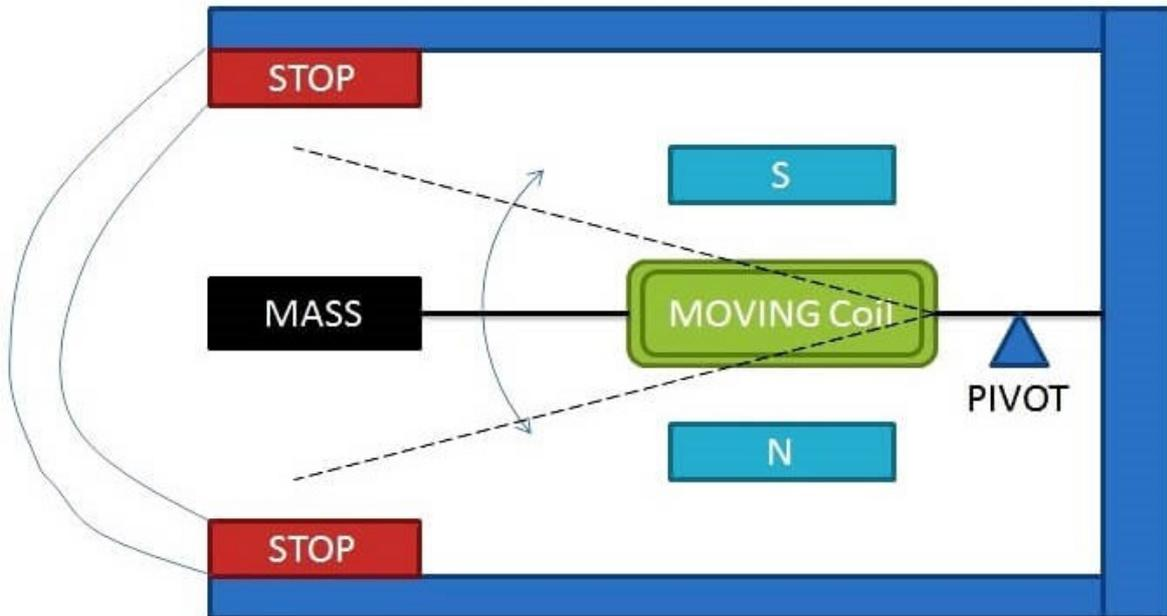
Figure 5.4: Element Of A Velocity Transducer.
