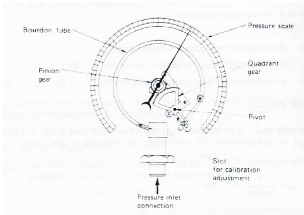
Figure 5.5: A Bourdon-Tube Pressure Gauge.
