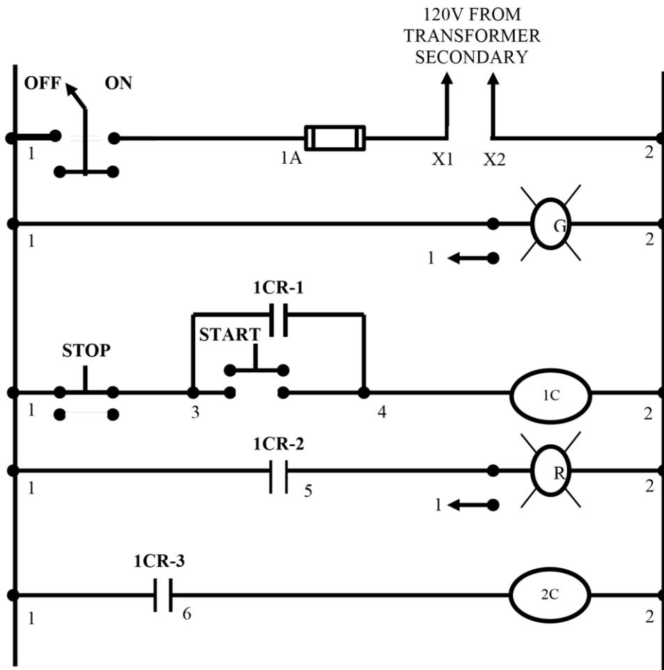
Figure 3.5: Addition of a selector switch, fuse, pilot light and a second relay.
