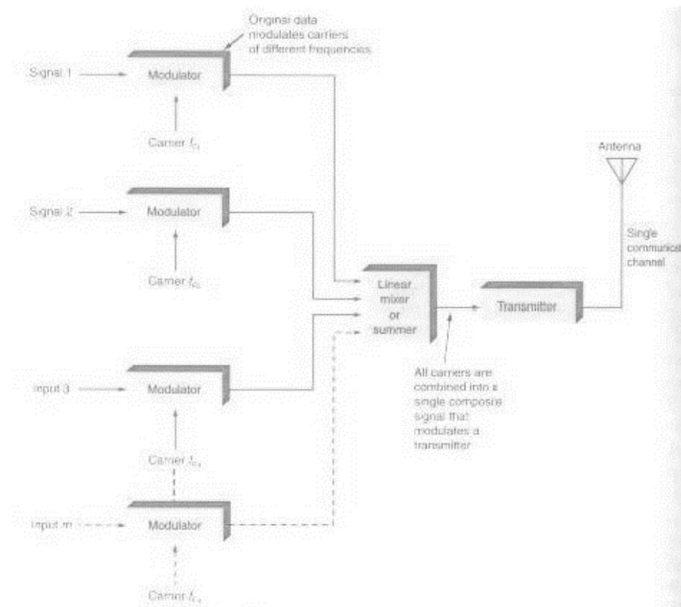
Figure 6.4: The transmitting end of an FDM system.
