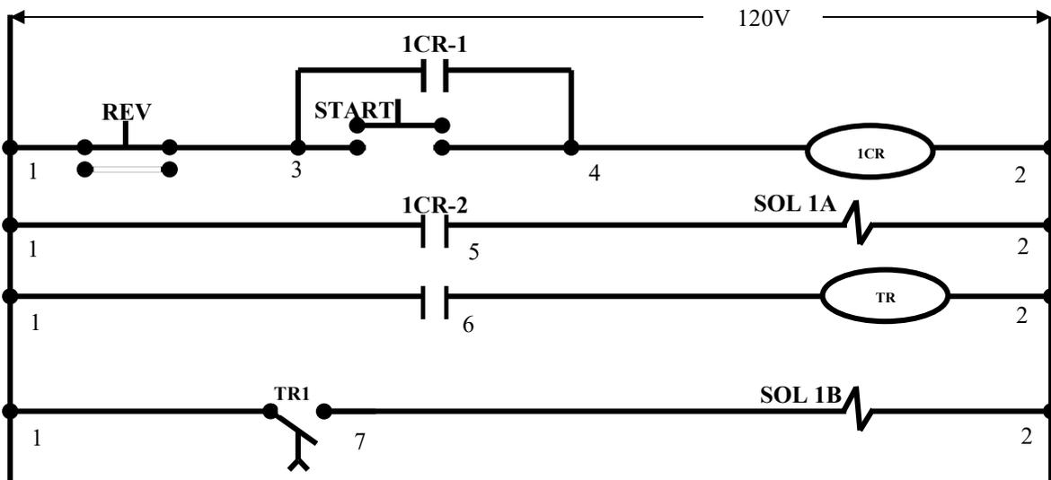
Figure 4.5: Single Solenoid Spring Return Valve.
