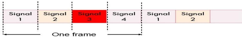
Figure 6.6: The basic TDM concept
