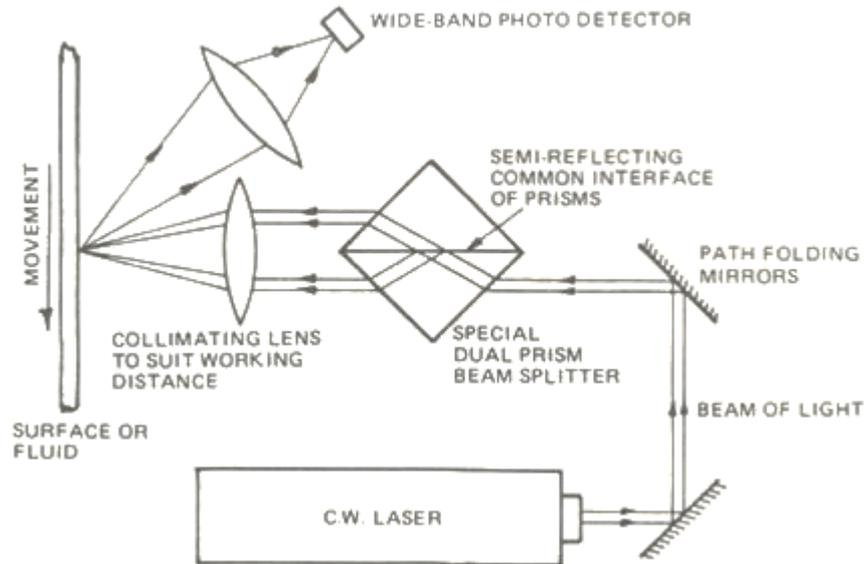
Figure 5.14: Laser Velocimeter.
