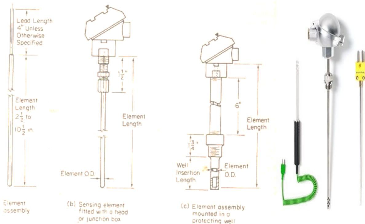
Figure 5.8: Resistance Thermometers.
