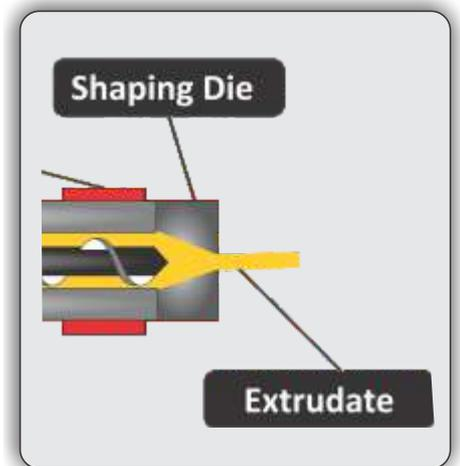
Figure 2.4 the die will take shape as is the shaping die
