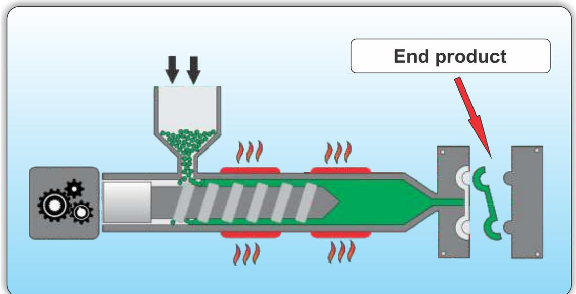
Figure 2.10 Step 4 of extrusion process
