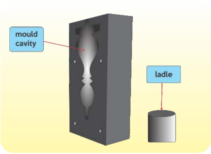
Figure 2.22 Example of mould cavity and ladle need for basic casting
