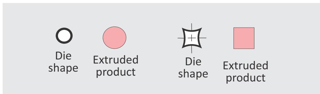
Figure 2.1 Common extrusion die geometries
