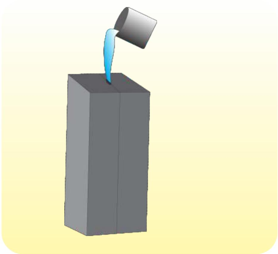
Figure 2.23 liquid plastic being pored into mould cavity
