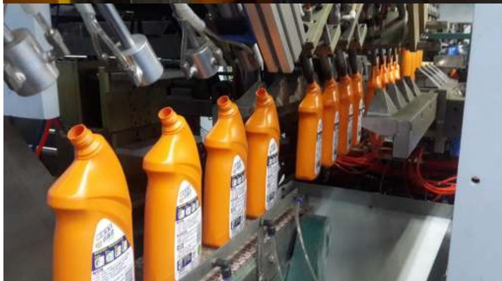
Figure 2.12 Example of blow moulding product.
