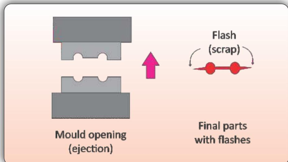
Figure 2.19 *The mould opening (ejection)*
