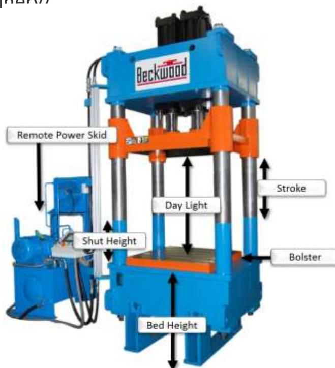
Figure 2.16 Compression moulding machine
