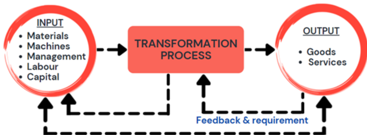
Figure 7: Basic block diagram in Production system
