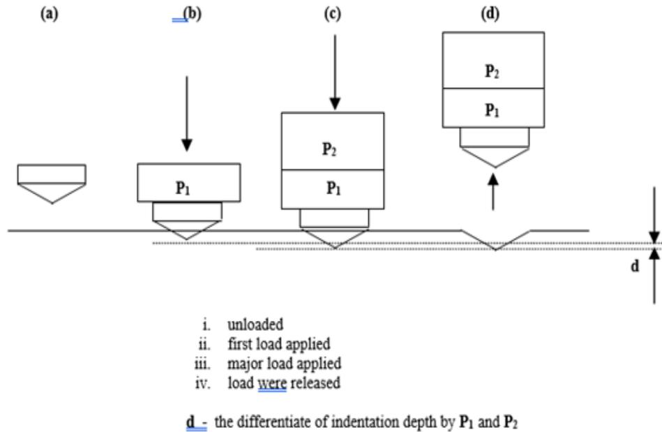
Figure 3.2: The principle of this Rockwell hardness test which is comparing the difference of depth of penetration of the indenter when using forces of two different values.
