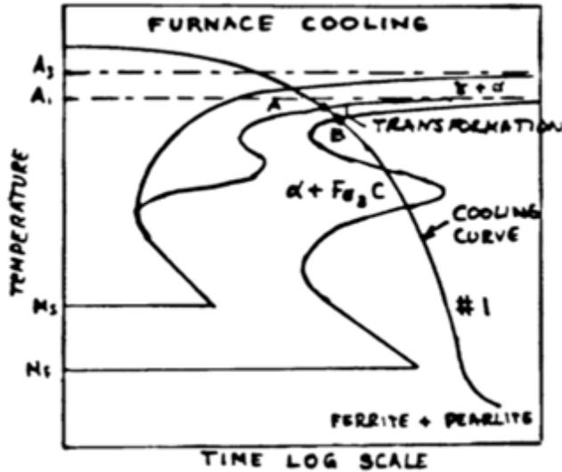
Figure 2.4: Typical TTT curve for a steel
