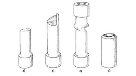
Figure 2 Failure patterns in torsion test
