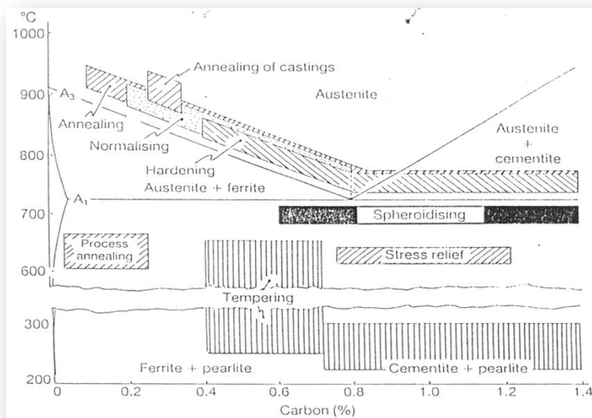
Figure 2.1 : Heat treatment for steel phase diagram
