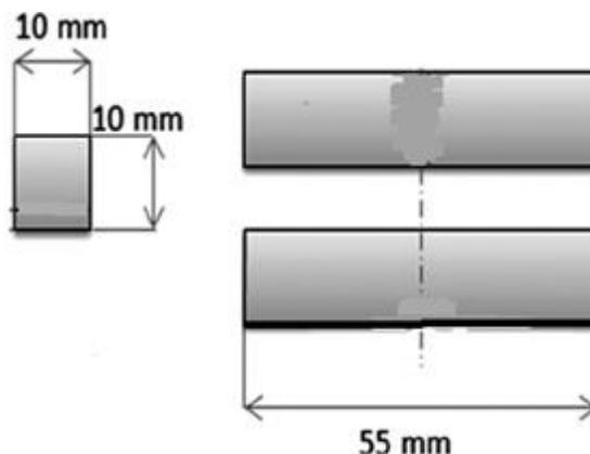
Figure 2.3: Dimension of specimen
