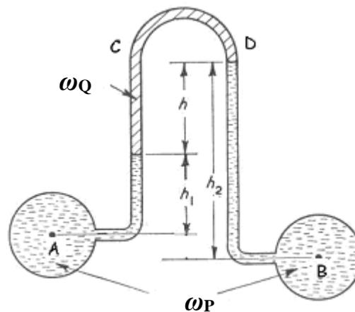
Figure 25: Inverted Differential Manometer
