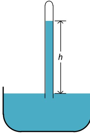
Figure 22: Mercury Barometer
