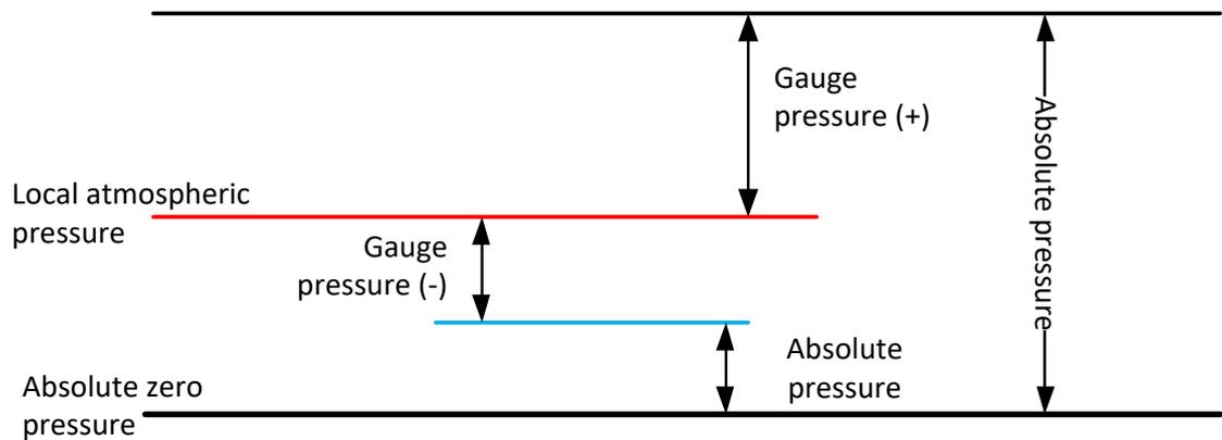
Figure 6: The relationship between Absolute and Gauge Pressure
