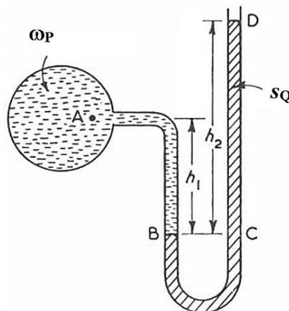
Figure 23: u-tube manometer
