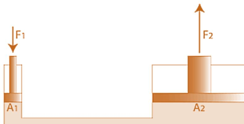
Figure 20: Schematic diagram of hydraulic jack
