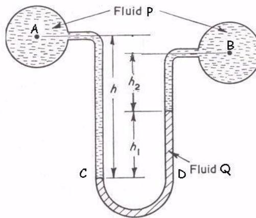
Figure 24: Differential Manometer
