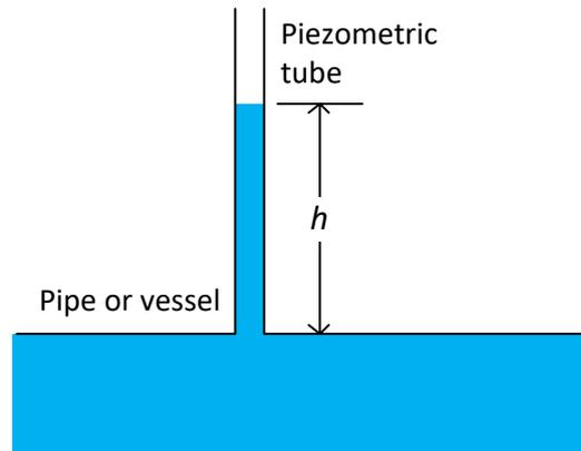
Figure 21: Piezometer inside a pipe
