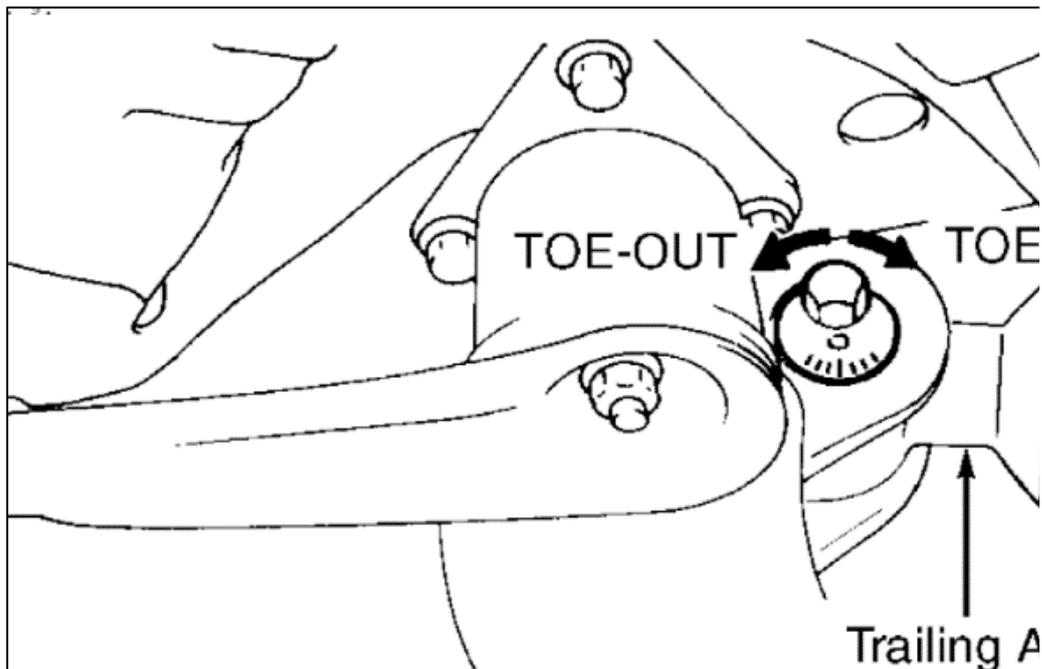
**Figure 11** : Location for adjusting toe angle
