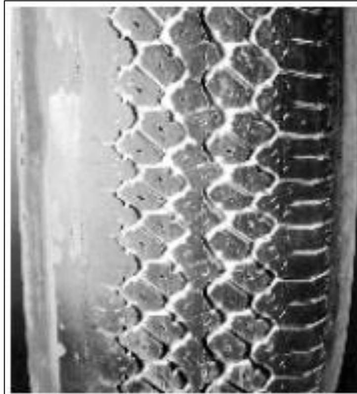
**Figure 5: Tyre Wear On One Side**
