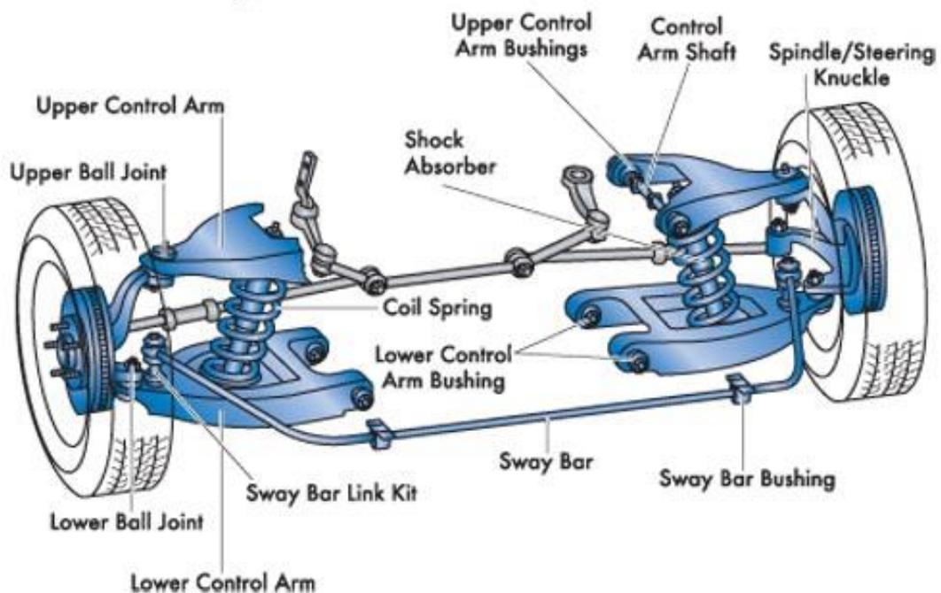
**FIGURE 1:** Suspension System
