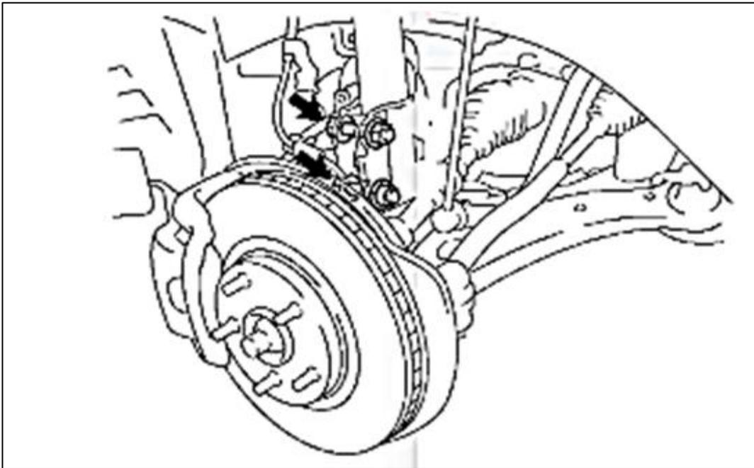
**Figure 11** : Replace knuckle nut with camber bolt
