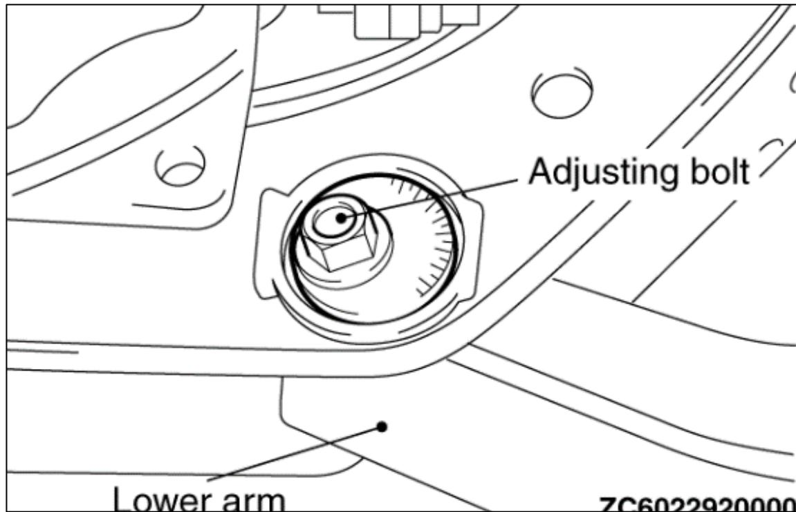
Figure 10: Adjusting bolt for rear camber
