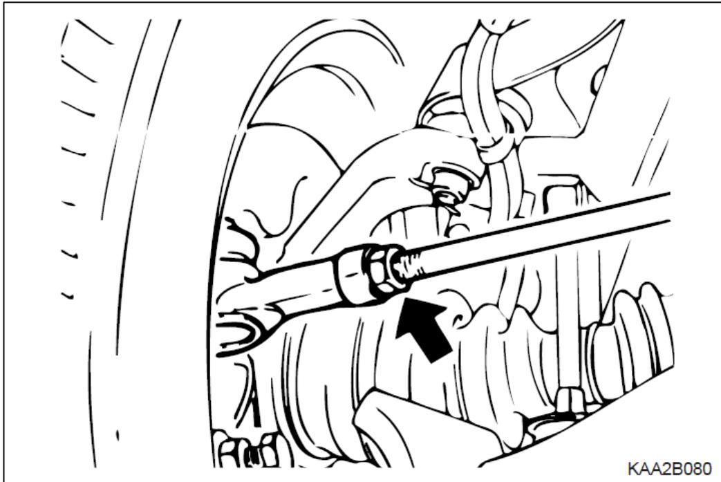
**Figure 12 :** Loosen the tie rod end lock nuts to adjust toe angle
