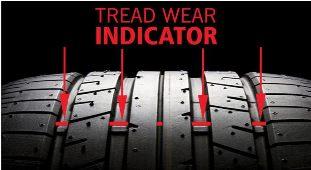
Figure 9: Thread wear indicator
