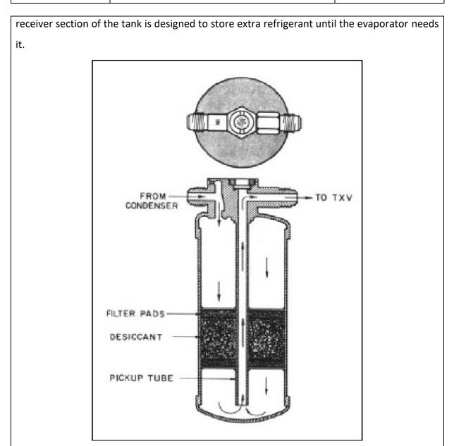
Figure 12: Receiver Drier
