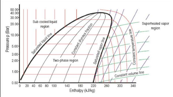
Figure 5: Skeleton of Pressure-Enthalpy Diagram.
