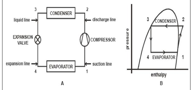
Figure 4: Vapor Compression System Schematic and refrigeration Cycle pressure-Enthalpy Diagram
