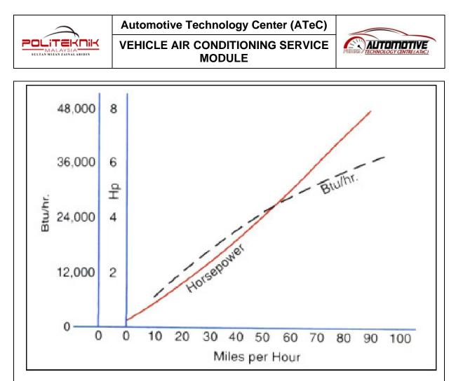
Fig. 3: Curves show relationship between car speed, heat load, and horsepower required to drive air conditioning system.
