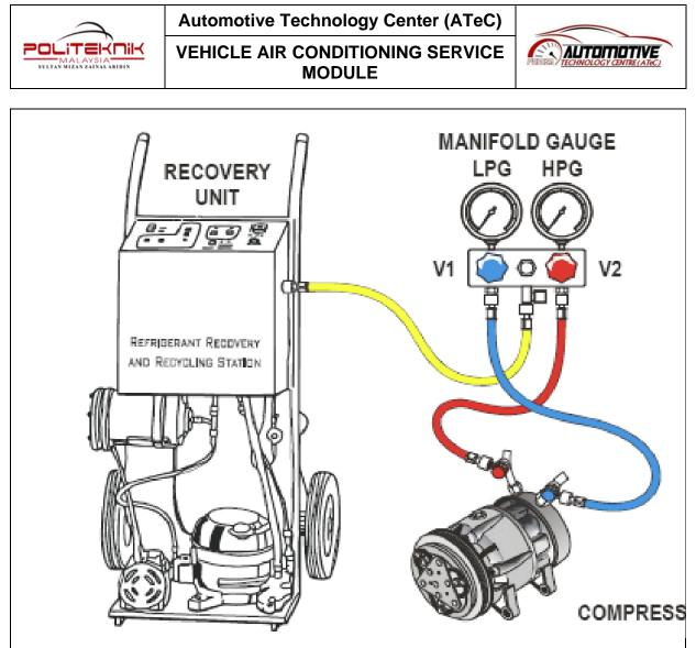
Figure 18: Connecting recovery unit to manifold gauge.
