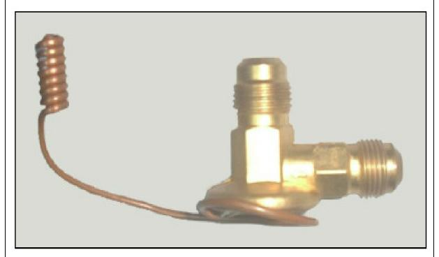
Figure 13: Thermostatic Expansion Valves.
