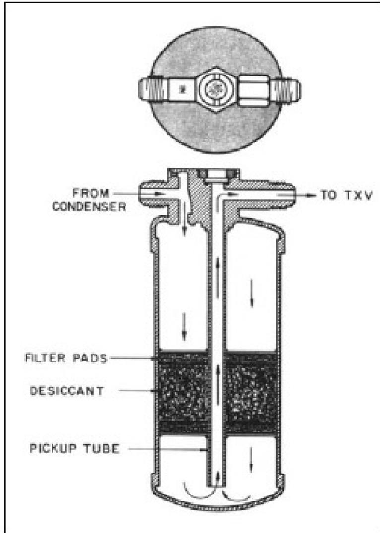
**Figure 12: Receiver Drier**
