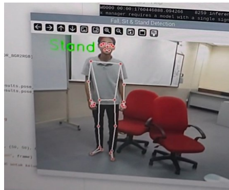
Figure 2. Real-time skeletal key point extraction and posture classification of standing
