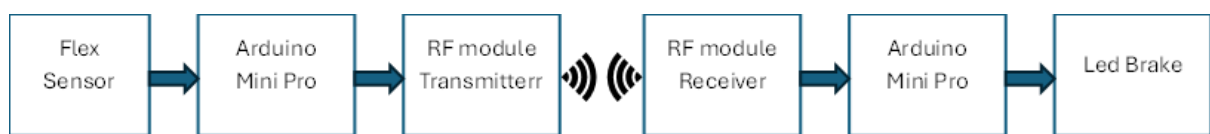
Figure 1: Operational block diagram for Smart Glove System for Bicycle Hand Signaling
