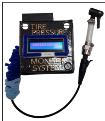
Figure 3: Prototype of Tire Pressure Monitoring System
