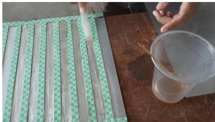
Figure 2: Preparing sample by hand lay-up method
