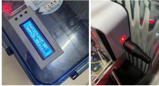
Figure 9 (b): Heater turns on when humidity above 50%
