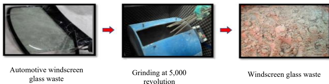
Figure 1: Preparation of automotive windscreen glass waste powder (WGWP)
