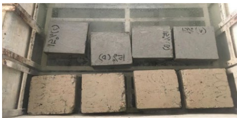
Figure 7: Conducting water absorption curing
