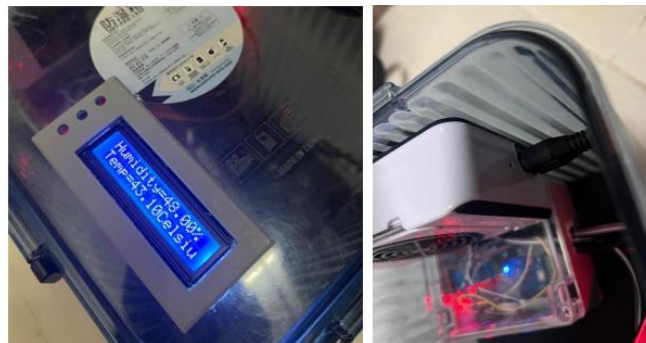
Figure 9 (a): Heater turns off when humidity below 50%
