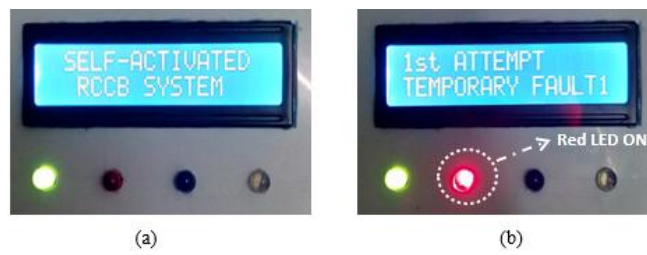
Figure 10: The Red LED - (a)Before Active, (b)After Active
