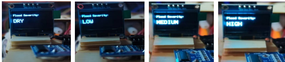
Figure 6: OLED Display Showing the Four Flood Severity Levels
