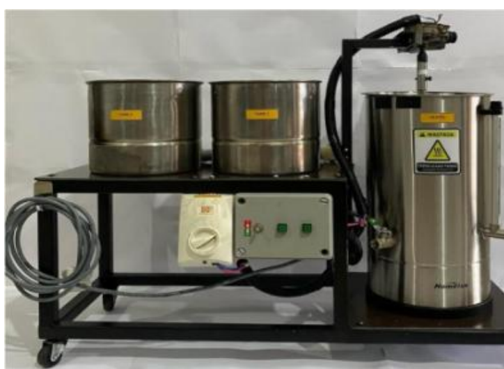
Figure 3 : WCO Biodiesel transesterification processing reactor (Azmi et al. , 2023)
