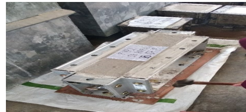
Figure 4: Mould with concrete admixture sampling
