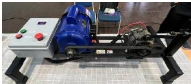
Figure 6: Main parts of alternator test bench
