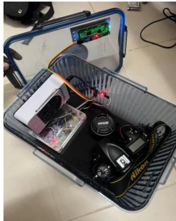
Figure 8 : IoT-based Humidity controlled Storage Hardware
