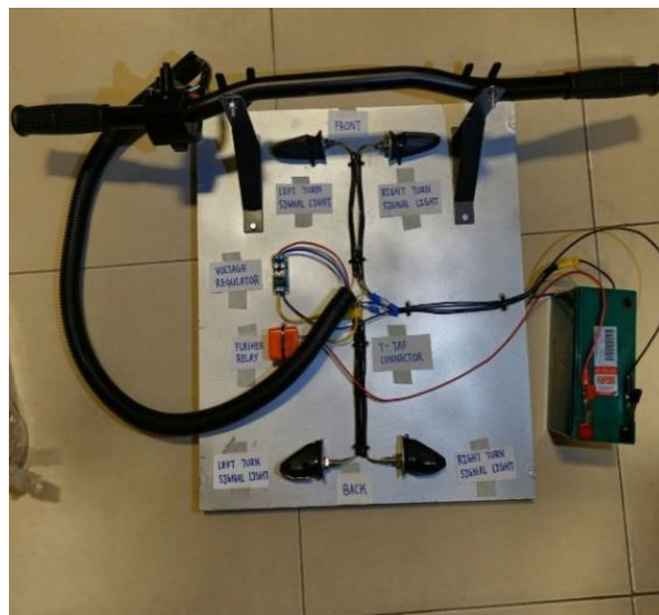
Figure 1: Turn Off Signal Alert System Prototype.
