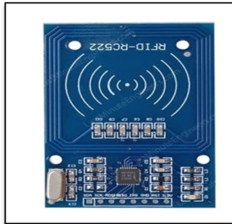
Figure 2: RFID module based on MFRC522 IC from NXP
