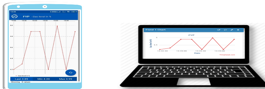
Figure 11: Gas concentration value map in ThingView and ThingSpeak
