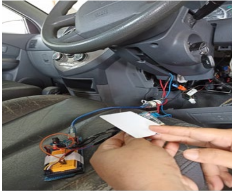
Figure 12: When wrong RFID card attach, the car not turn on
