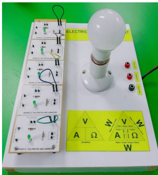
Rajah 8: Papan Pengukuran Elektrik - Electrical Measurement Board (EMB)
