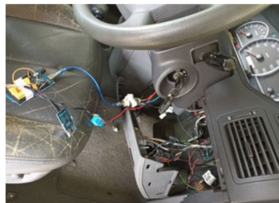
Figure 11: Complete circuit install in car ignition system
