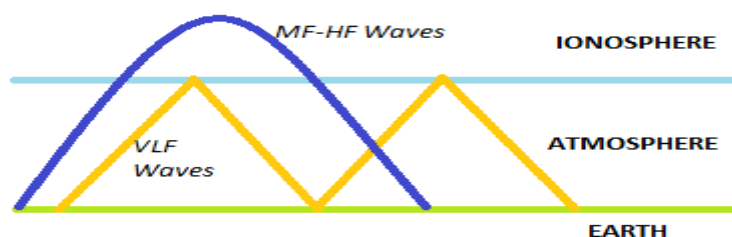
Figure 1: The Earth's ionosphere propagation and reflecting of VLF radio waves
