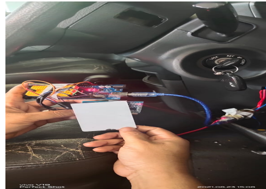
Figure 13: When correct RFID card attach, the car will turn on
