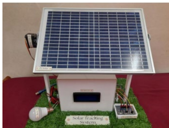
Figure 3: Solar Tracking System (STS)
