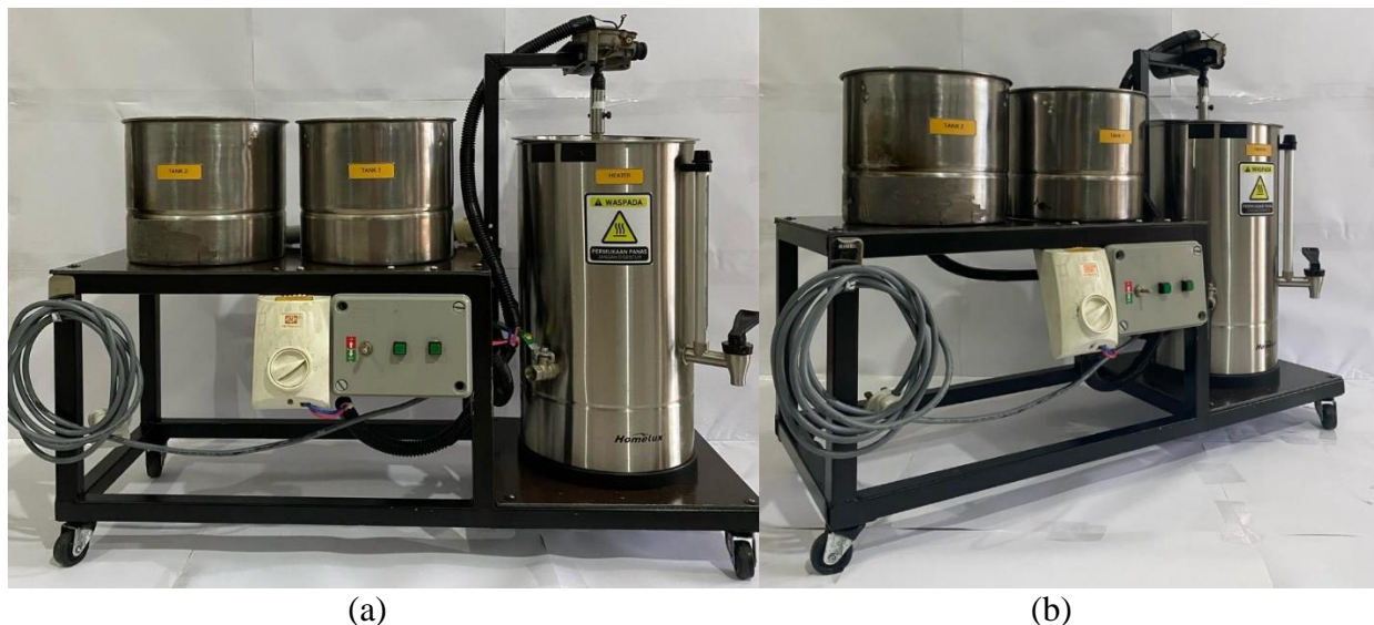
Figure 5: WCO Biodiesel Processing Reactor; (a) Front view, (b) Isometric view
